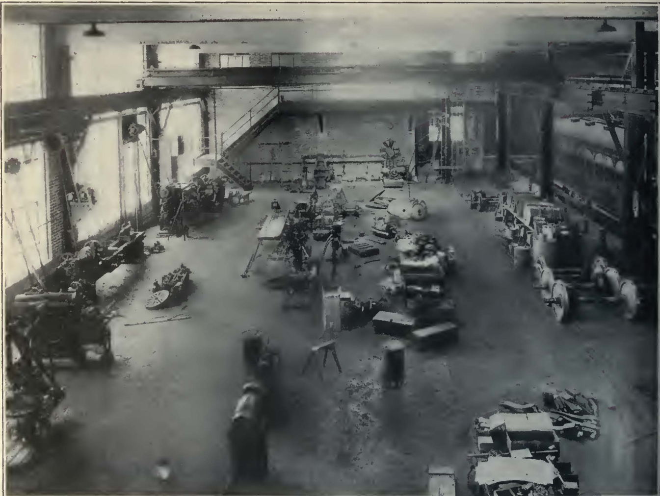
Materials Are Handled in the Machine Shop by a 5-Ton Electric Crane Operated from the Floor
