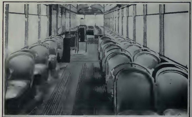
Bucket Type Leather-Upholstered Seats Being Tried on One Two- Car Train of the Cleveland Railway Have Proved Very Popular
