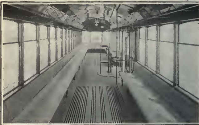
Looking Forward in a Standard Trailer Used in Cleveland, Showing Seating Arrangement
