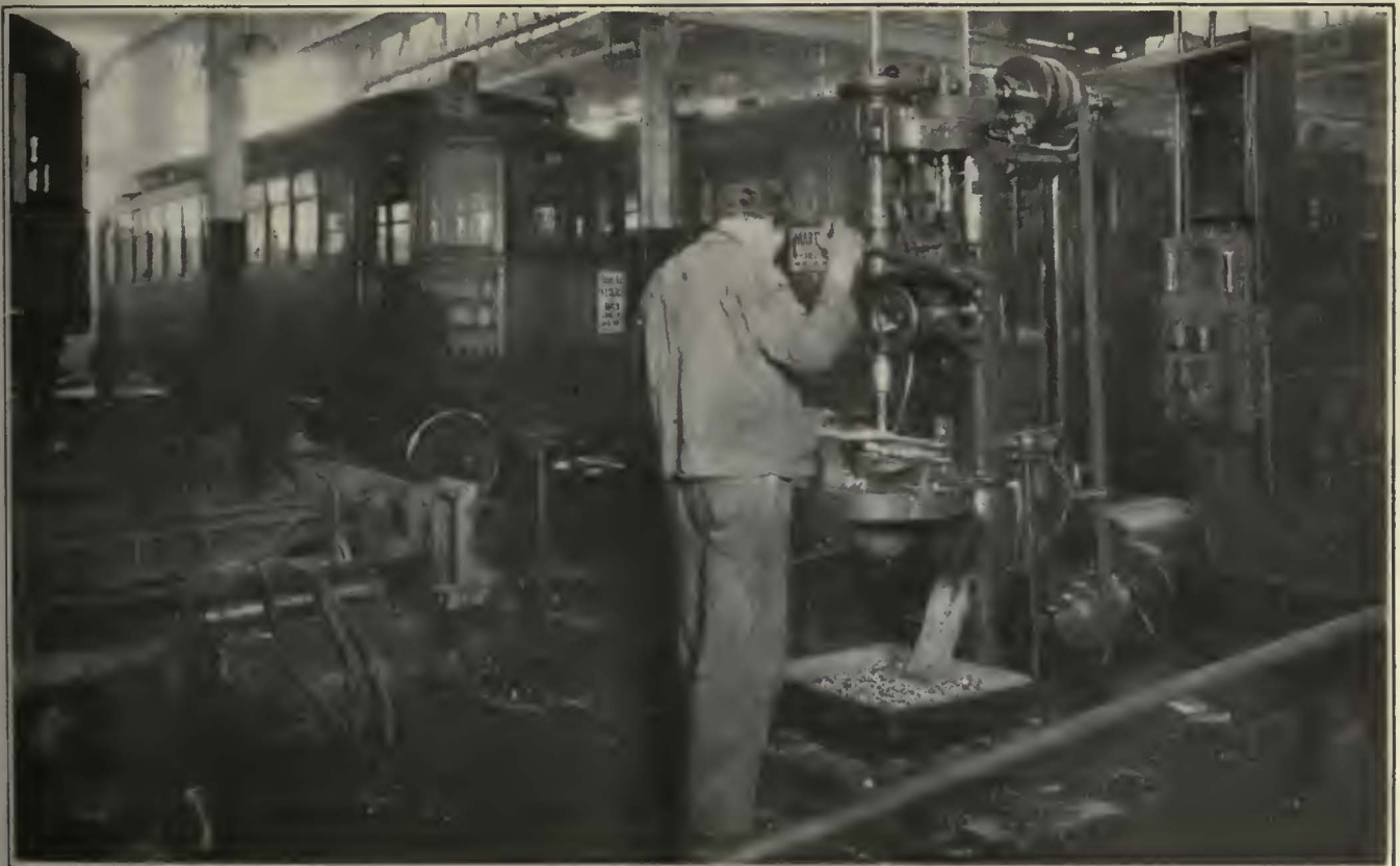
Drilling a Truck Hanger in the Overhauling Shops of the Department of Street Railways, Detroit
