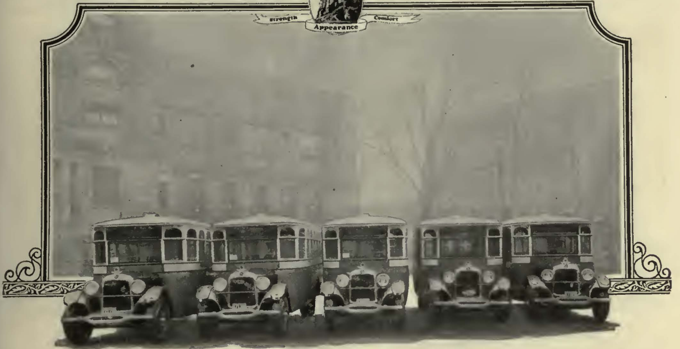
Twenty-one passenger street car type Studebaker busses for South Bend Indiana Railroad
