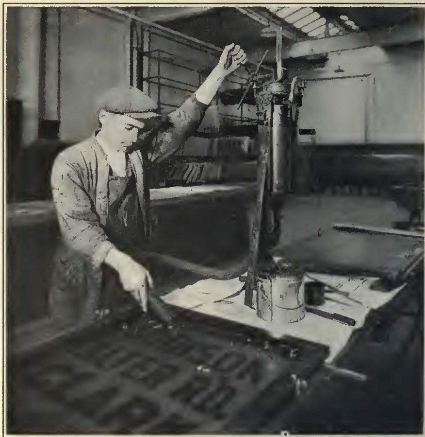
Thick Paint for the Silk-Screen Process Is Supplied to the Screen by a Press Can and Flexible Hose Attachment in the Department of Street Railways, Detroit, Mich.
