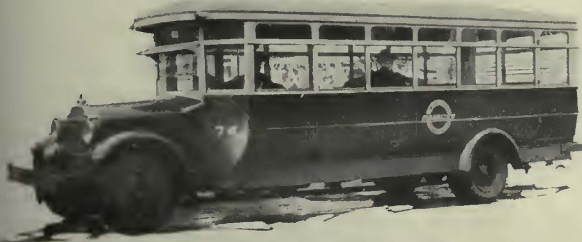
A Mack Gas-Electric Bus in service. Note the generous ground clearance—0½ inches.
