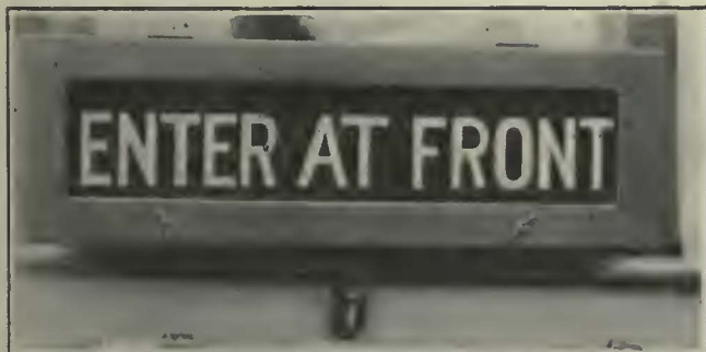
Close-Up of Front Sign Reading "Enter at Front." This, as Well as Interior Signs, Is Turned on by an Air-Operated Switch Attached to the Brake Line, so It Is Illuminated Only When Brakes Are Applied
