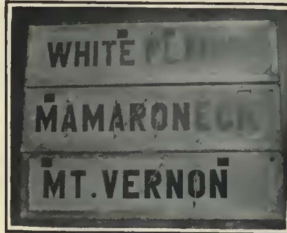
Lead Stencils with Loose Parts Held in Place by Wires Raised from the Surface
