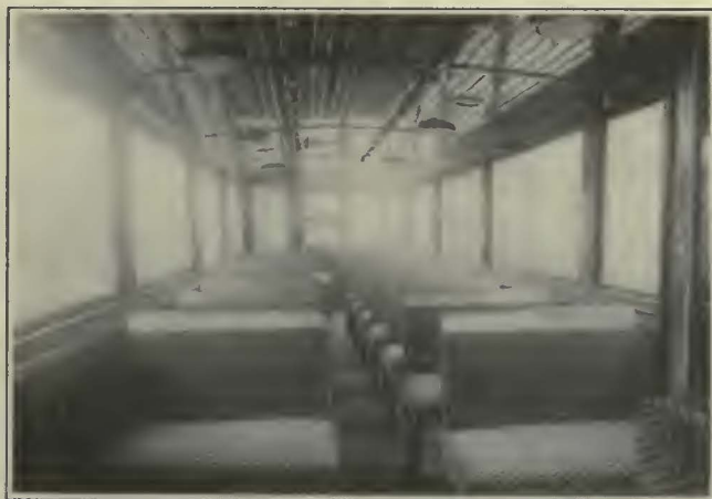
Seats and Backs on the Upper Deck of the West Ham Car Are Spring-Cushioned and Attractively Upholstered
