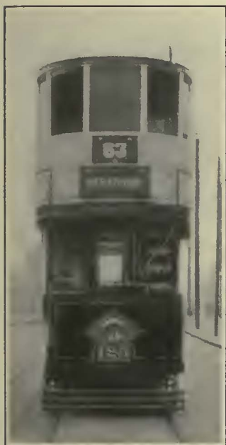
New Car of the West Ham Corporation Tramways Is One of a Comparatively Small Number of Double-Deck Vehicles Included in Recent British Orders. At the Left Is the End View of This Car, Showing Collision Bumper That Is Backed Up by Strong Spiral Springs
