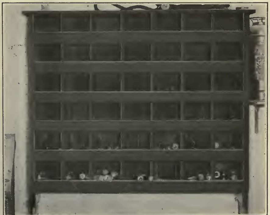
A Rack for Keeping Bolts Handy to Truck Overhauling Work Has Been Found Useful in the Shops of the Grand Rapids Railway
