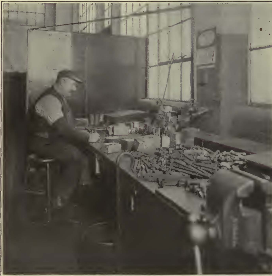
General Salvage Man in the Department of Street Railways, Detroit, Sorting Machine Screws and Placing Them in Proper Boxes
