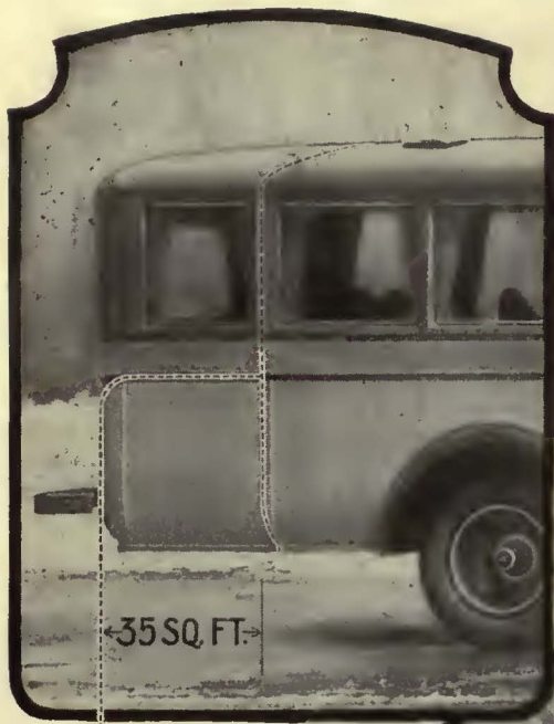
A 25-passenger bus equipped with the Baker-Raulang Luggage Loft carries 30 paying passengers, with no increase in wheel-base.
