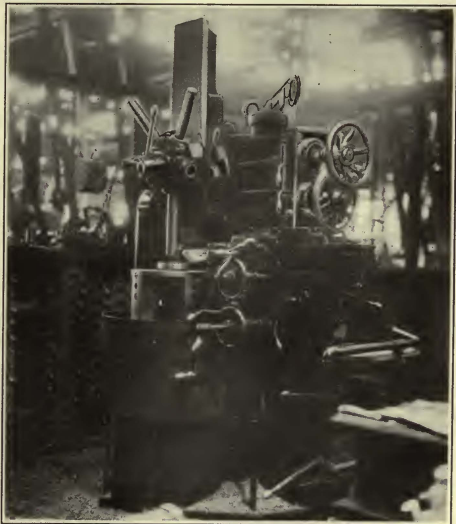
Bullard Vertical Turret Lathe for Machining Split Bearings
