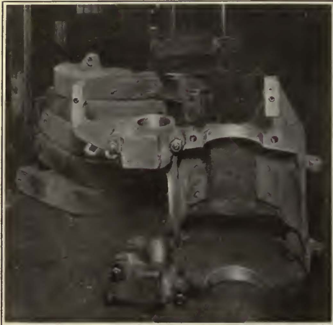
The Upper Half of a Westinghouse 101-B Split Frame Motor and Axle Caps After Being Welded and Rebored
