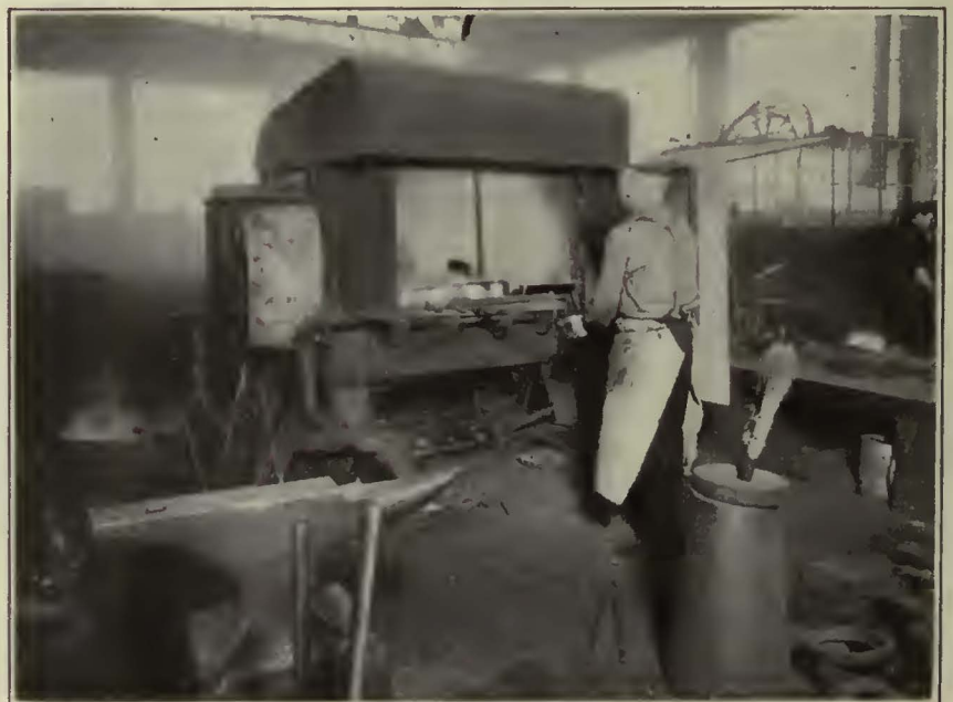
Heating Plects Preparatory to Repointing in One of the Oil-Fired Furnaces
