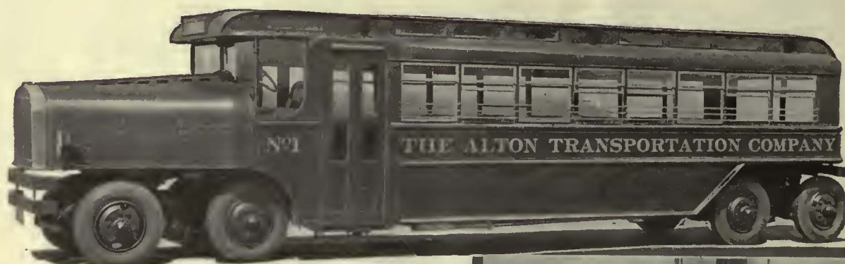
Versare-Westinghouse Coach for Chicago & Alton R.R. Equipped with Edwards Metal Sash, in windows, deck lights and windshield. Note the clear vision afforded.
