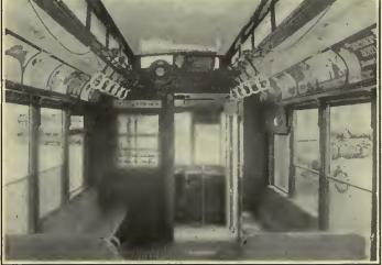
The Interior View at the Left Shows the Arrangement of Seats, that at the Right the Method of Tapering One Longitudinal Seat at Each End to Provide a One-Piece Door with 37-In. Opening
