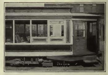
The Platforms Are Supported on Knee Plates Bolted to the Side Sills. A\*Platform Can Be Removed by Taking Out Five Bolts on Each Side
