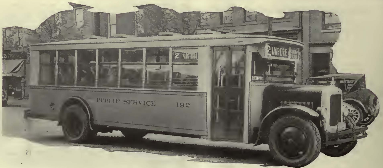
A Comparatively Flat Roof and Windows with Stationary Upper Sash Are Features of the Benedict Body Built in the Railway Shops
