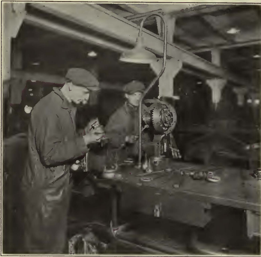
Efficient Bench Lighting as Provided in the Shops of the Department of Street Railways, Detroit
