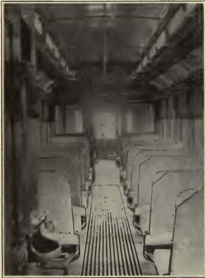
Bell Cord, Baggage Racks, Ventilator Operating Rods, Etc., Cluttered Up the Interior of the Old Car
