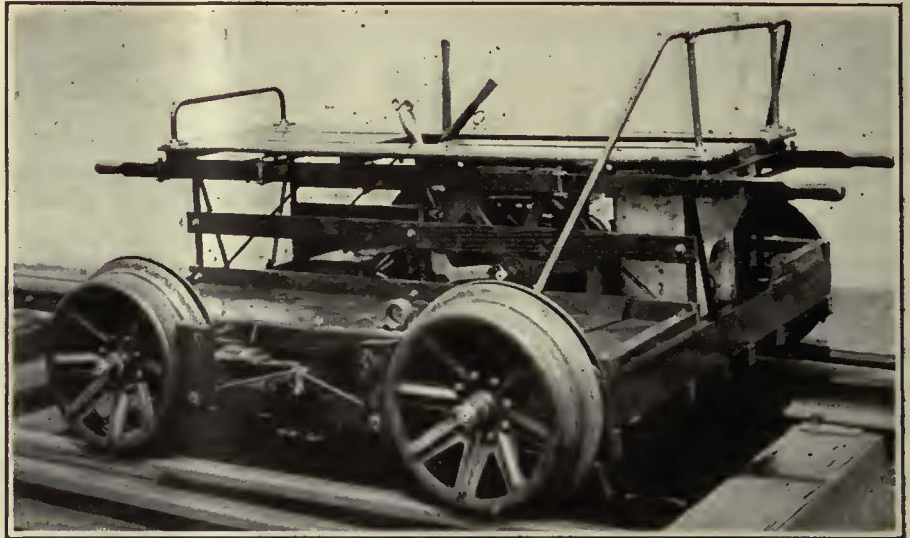
View of the Mudge Inspection Car, Showing the Self-Equalizing Brake Equipment
