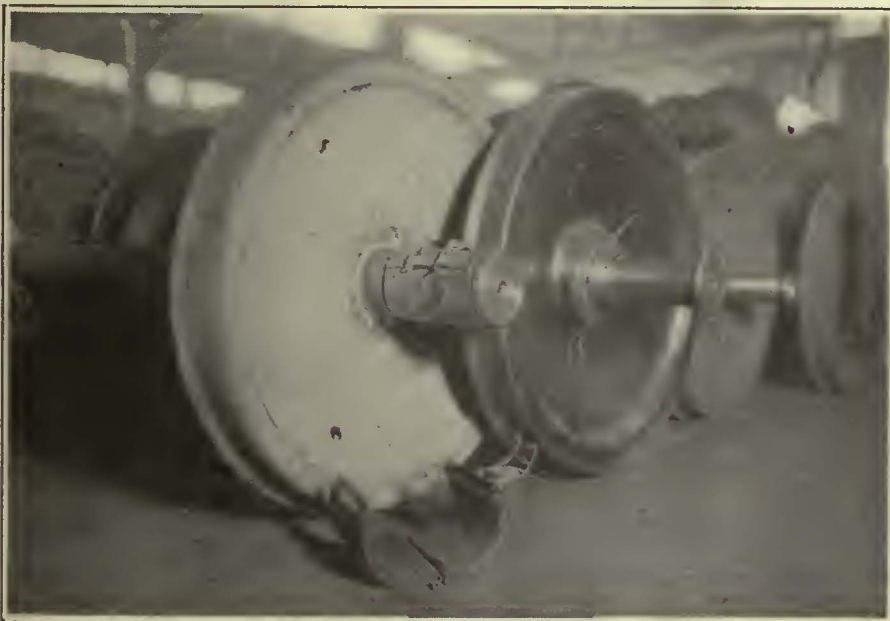
A Special Fixture Placed Around the Journal Prevents Damage from the Flanges of Adjacent Wheels
