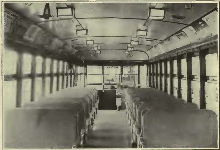
Interior of the New Twin City Car, Showing Type of Lighting Fixtures Used
