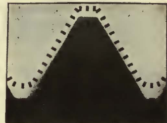
Comparator photograph showing profile of thread of an Empire New Process Bolt.
