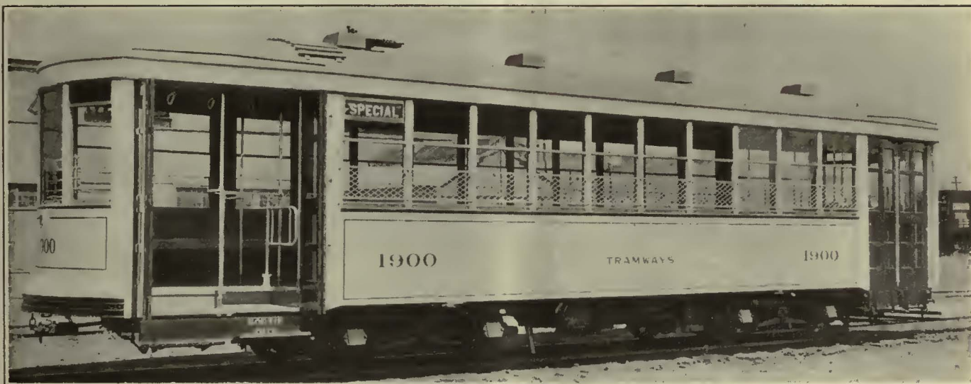
Each Platform of These Cars Has a Door for Entrance and a Door for Exit, but the Rear Door on the Rear Platform Is Used Only with Two-Man Operation
