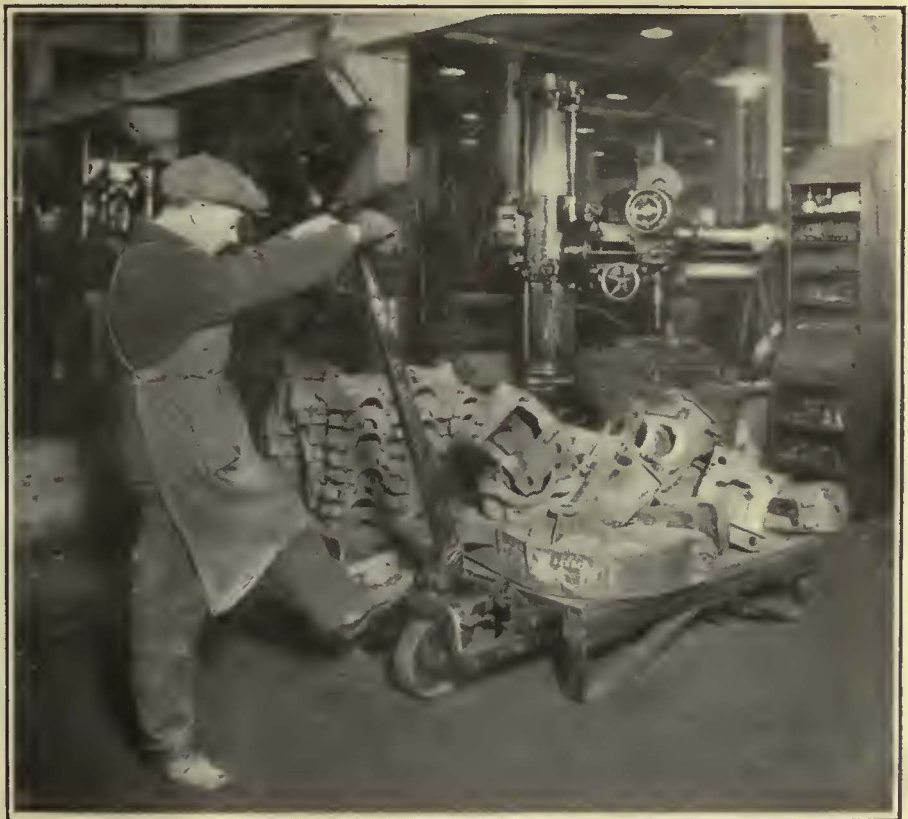
Hand Trucks with Separate Platforms Are Used for Moving Heavy Parts About the Shops of the Department of Street Railways, Detroit, Mich.
