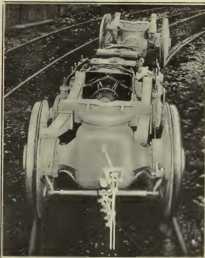
End View of Trucks Showing Spring Supporting Arrangement for Car Body
