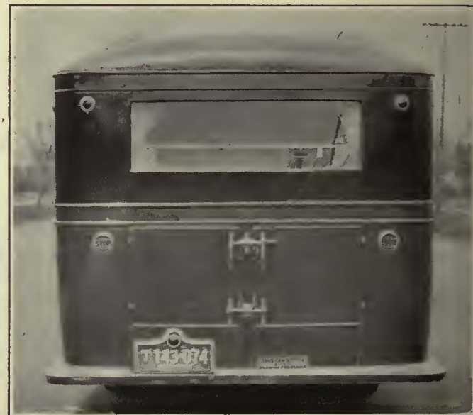
Doors in New Style Baggage Car Closed, and Ready to Move. Note the Recessed Aluminum Frame for the Tail Light and State License Plate
