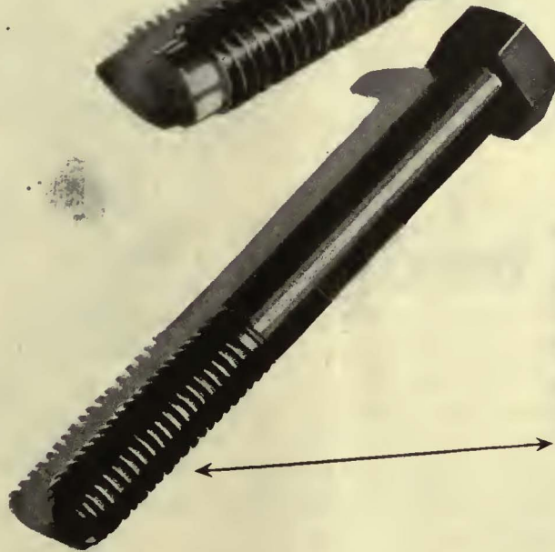
Comparator photograph showing profile of thread of an Empire New Process Bolt.
