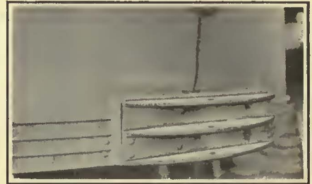
Combination Anti-Climber Bumper and Draw Pocket Installed at Center of Standard Anti-Climber
