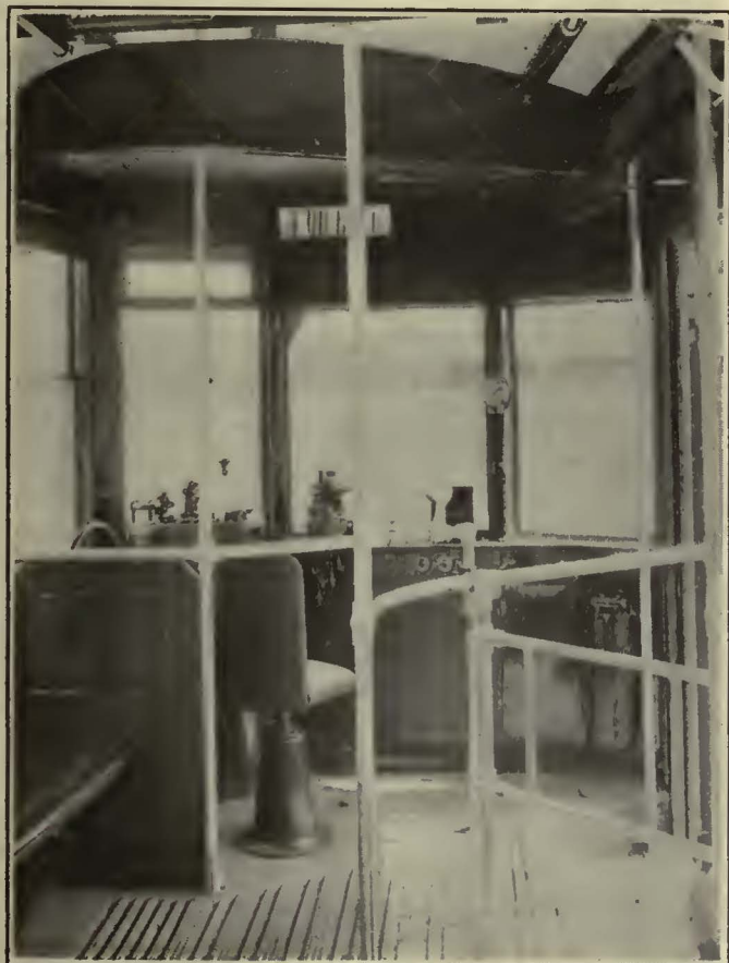
On the Front Platform All Piping Is Inclosed so as to Be Out of Sight. The Motorman Has a Comfortable Revolving Chair
