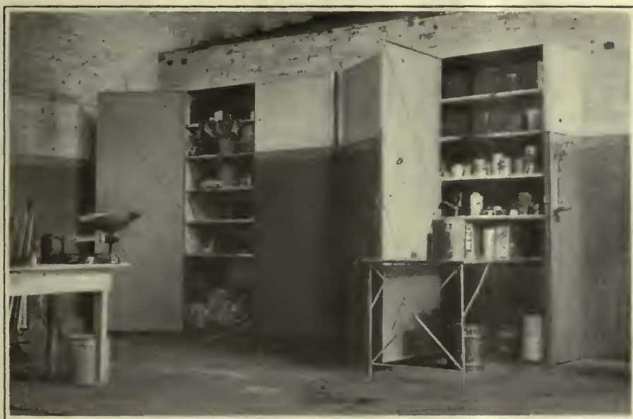
Steel Cabinet Built by the Chattanooga Railway Shop for the Storage of Paints and Oils in Use in the Painting of Cars
