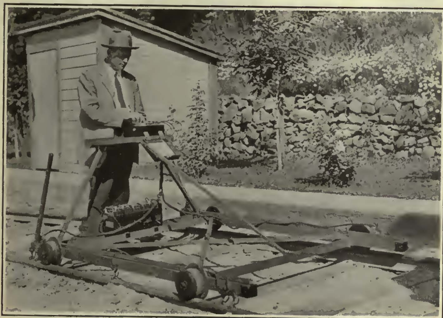
The Test Car Is Rolled Over the Joint to Be Tested and the Operator Takes a Reading on the Instruments
