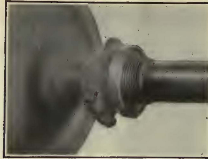
Loosening of Axle Collars Is Prevented on the Levis Tramways by Threading Them
