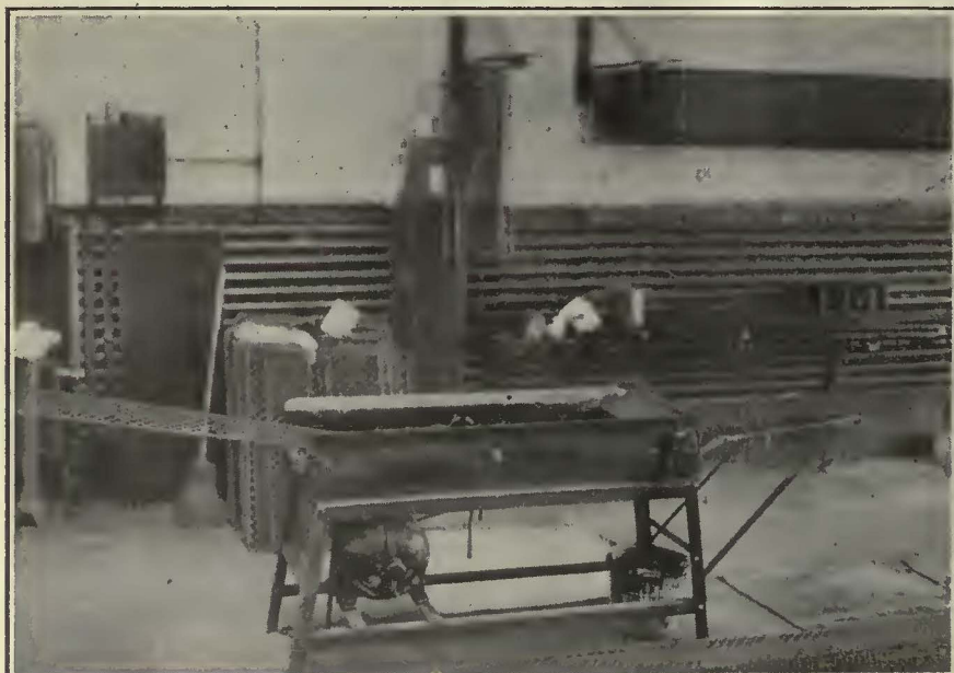
Window Guards Are Painted in a Few Seconds in the Cleveland Shops by the Use of This Paint Tank. As the Guard Emerges the Motor-Driven Brushes at the Right-Hand Side Thoroughly Brush the Paint into All Parts of the Guard and Remove the Surplus
