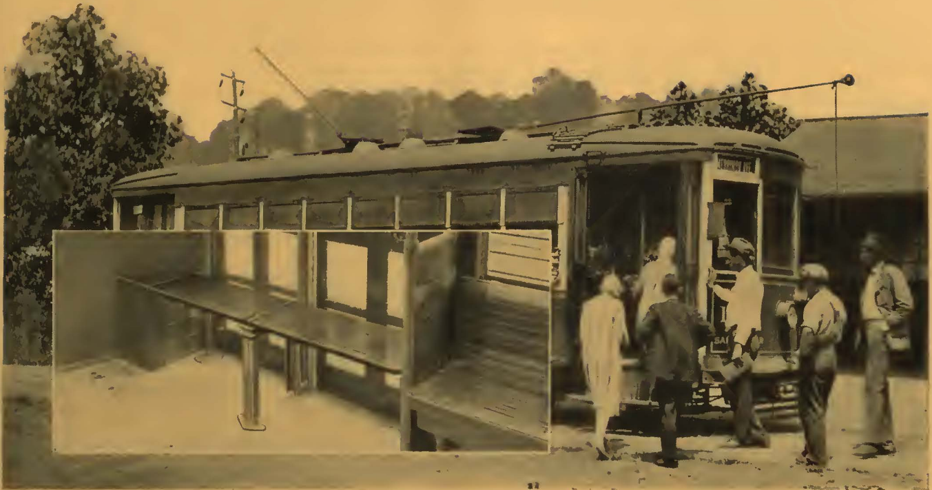
Seating capacity of Asheville's safety cars increased to 40 with Brill "Admor" Seats
