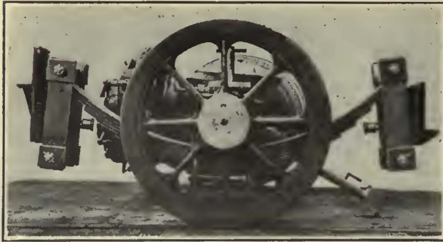
By This Arrangement of Springs the Unsprung Weight Is Kept Down to a Minimum
