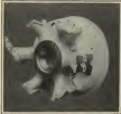
Rear Dual Wheel Showing Hub Spider with Brake Drum but Without Rims
