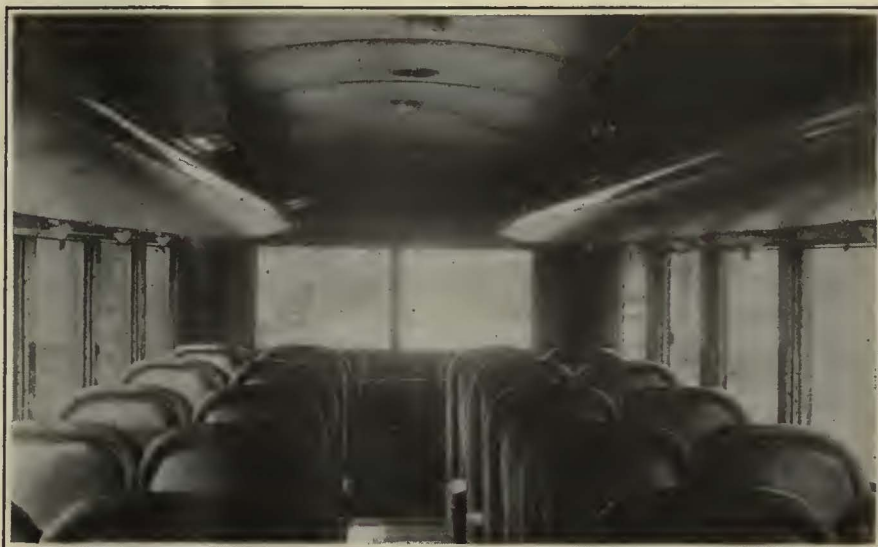
Improved Bus Construction Provides Folding Seats Across the Rear and a Combination Guide Rail and Luggage Loft
