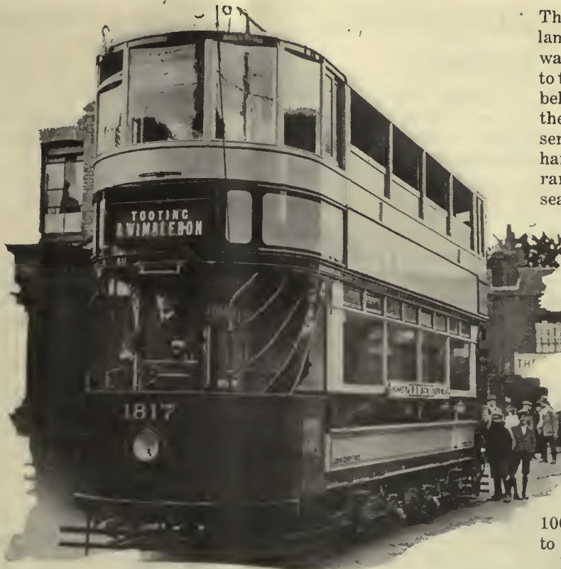
London County Council Tramways is Improving the Quality of its Service by Installing More Powerful Motors and Rearranging the Interior of Cars of This Type
