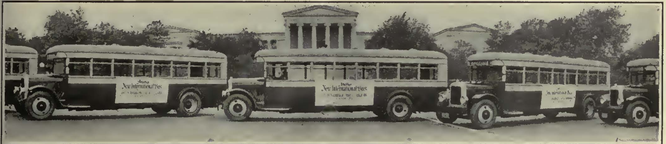
These Gas-Electric Buses Will Be Used In Interurban Service Out of Buffalo
