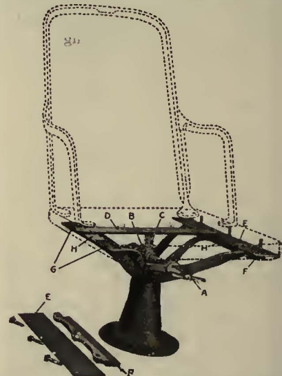
Adjustable Seat with Pedestal. The Seat for Mounting on Battery Box Is Similar in Style
