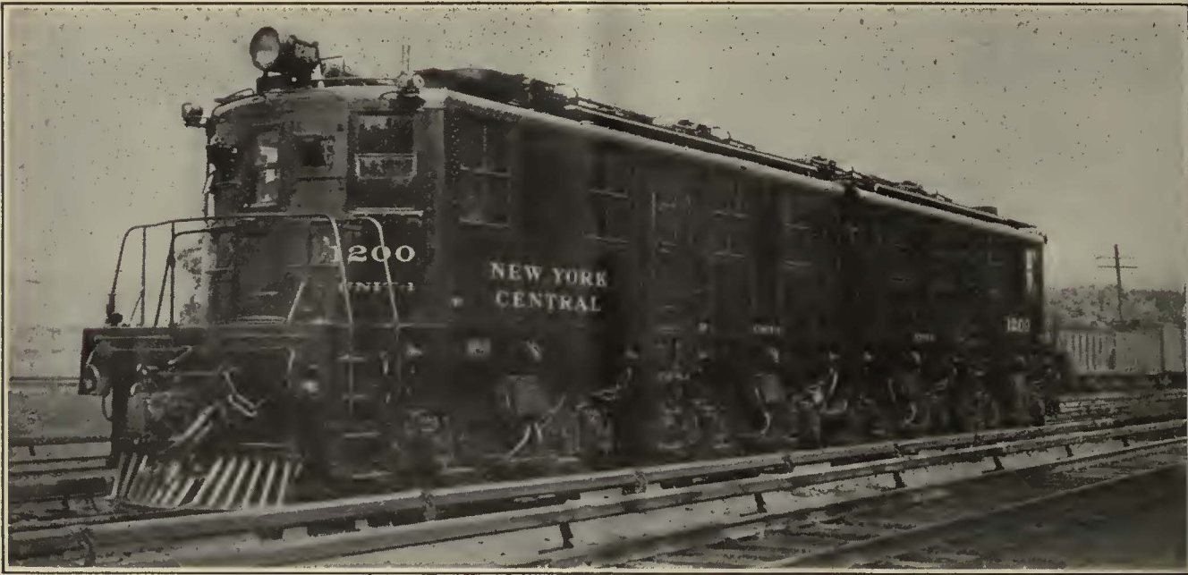
This Locomotive Pulled a Train of 108 Cars at a Maximum Speed of 32 M.p.h.
