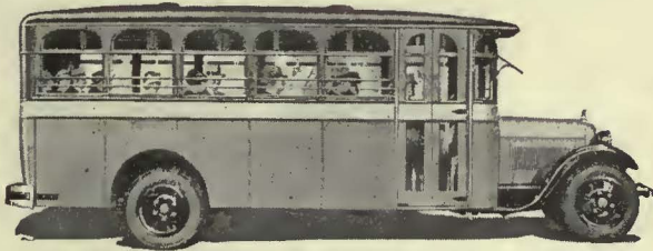
Studebaker 21-Passenger Pay-Enter Street-Car type bus (Dual Rear Wheels); $5125, f.o.b. factory. The most powerful bus chassis of its size in the world, according to the rating of the Society of Automotive Engineers
