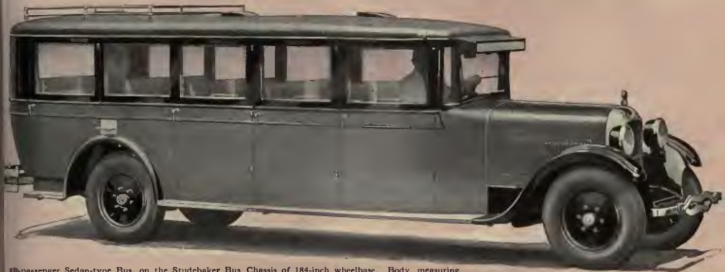
10-passenger Sedan-type Bus, on the Studebaker Bus Chassis of 184-inch wheelbase. Body, measuring 198 inches long and 76 inches wide, is distinctive in design and appearance. Lacquer finished in a choice of two color combinations. Four wide doors, also driver's door and an emergency door on the left. Cross seats or semi-chair type seats accommodate 19 passengers in comfort. (Also available in full-chair type for 15 passengers.) Completely equipped. The coupon below will bring further particulars.
