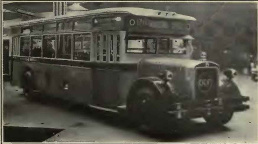
Easy Riding Qualities of This Six-Cylinder "a.c.f." Bus Are Enhanced by Long Springs
