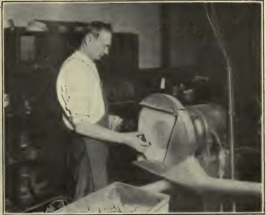
Removing the Barrs from Both Sides of the Individual Copper Bars by Grinding
