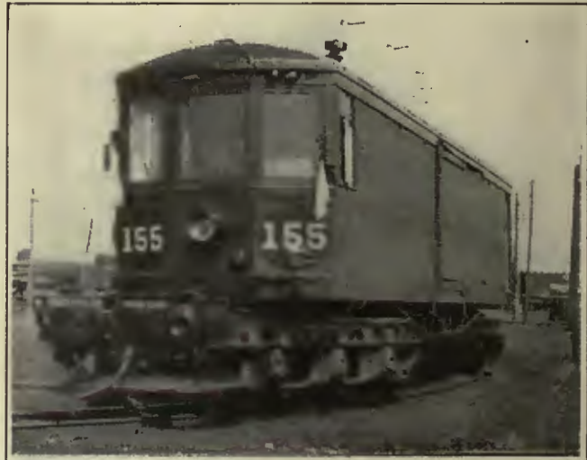
Freight Car of the Western Ohio Railway Equipped with Six Motors and Twelve Driving Wheels
