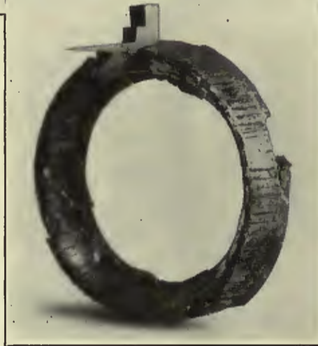
Hard-Drawn Copper Bar After Years of Service
