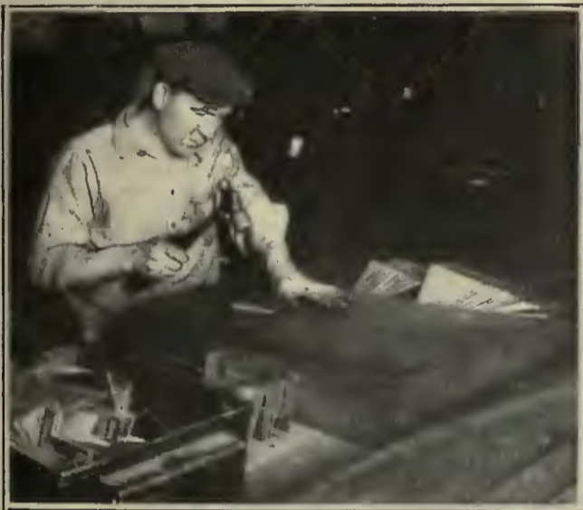
Copper Bars Being Straightened Before Building into an Assembled Set of Commutator Segments
