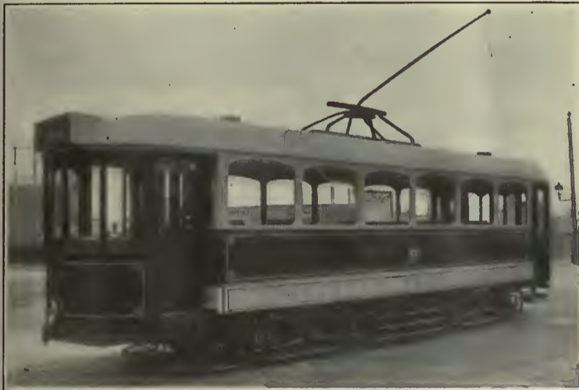
Many Features Characteristic of American Electric Railway Practice Are Embodied in the Design of This New Single-Deck Car of the Glasgow Corporation Tramways. At Right, Arrangement of Equipment on the Platform Follows the Usual American Practice
