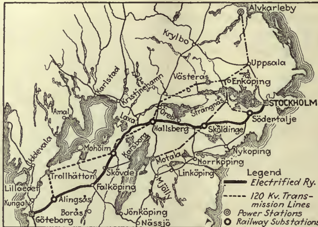
Map Showing Electrified Line, Generating Station and Substations
