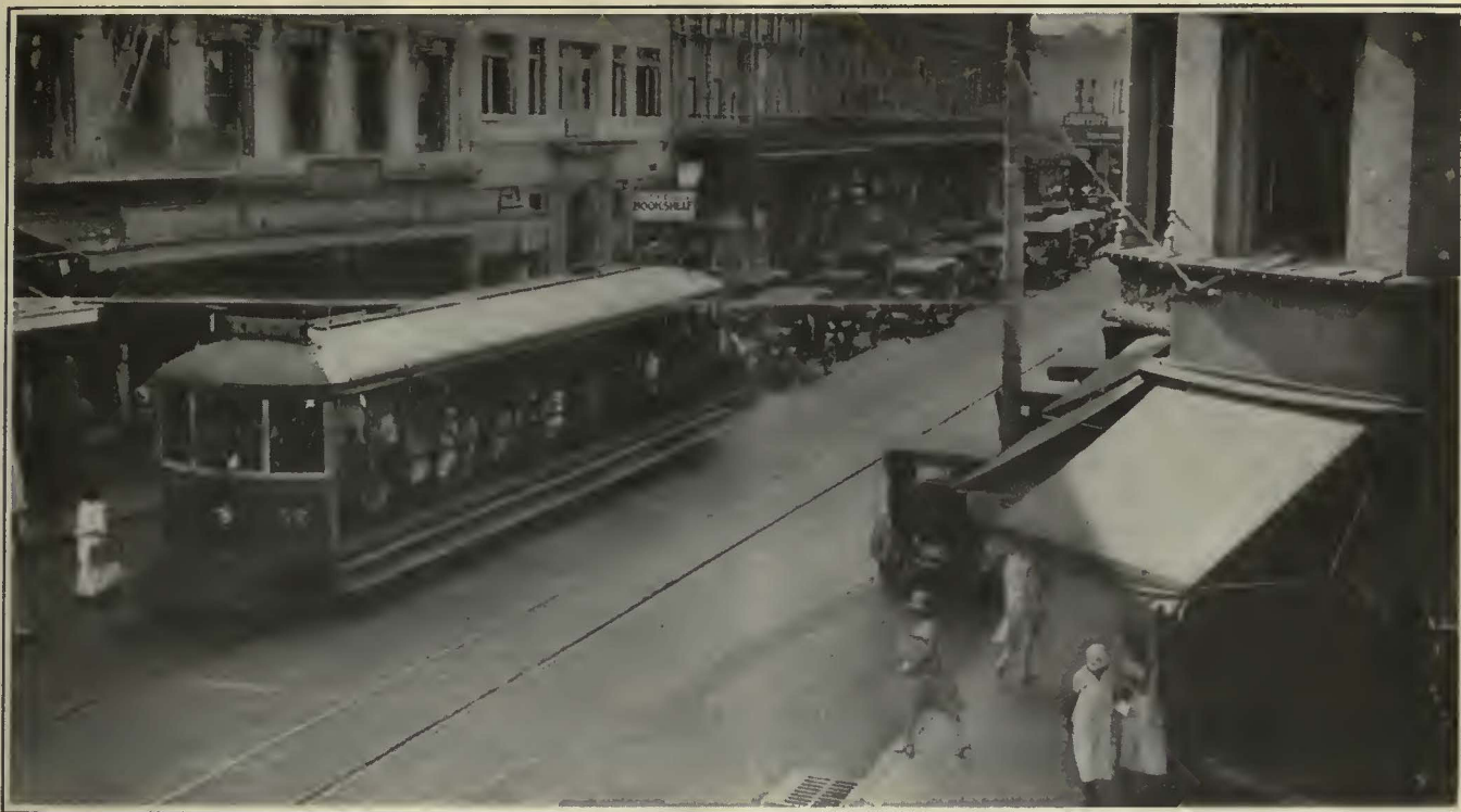
Latest Type Open Car of the Honolulu Rapid Transit Company with Center Aisle Has a Seating Capacity of 56
