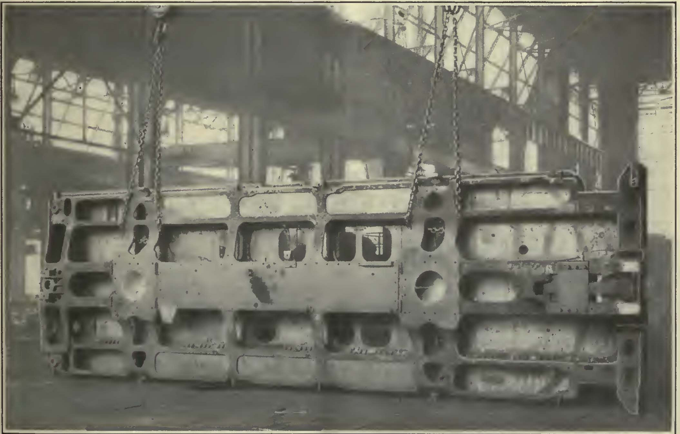
One of the innovations in this electric locomotive is the cast-steel floor frame type of construction. This eliminates an expensive assembly job using structural shapes and rivets
