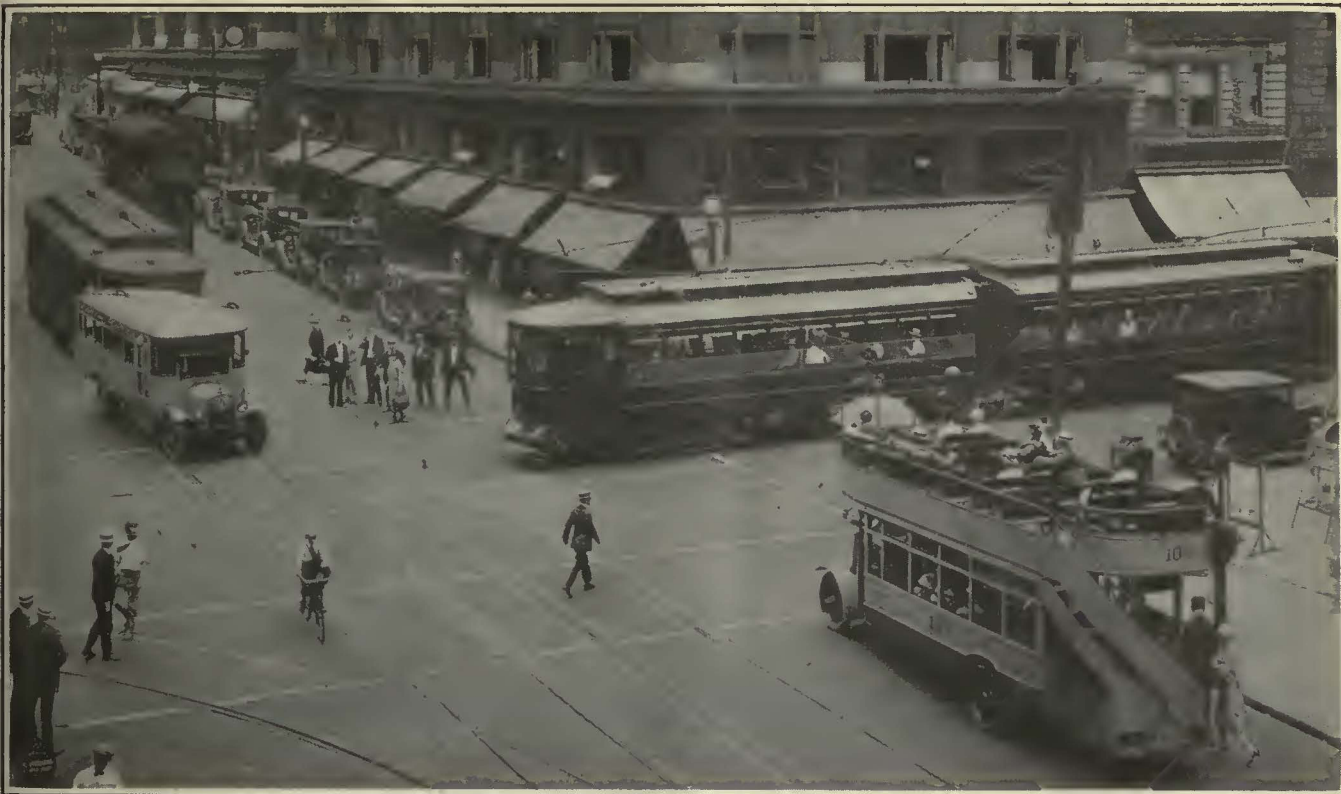
This View Shows an Articulated Car, a Single Car, a Single-Deck Bus, a Double-Deck Bus with Open Top and a Double-Deck Bus with Closed Top, All About to Make the Crossing at Sun Square, One of the Oldest and Busiest Cross Roads of Baltimore
