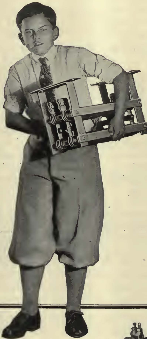
At right—3600-watt cast-iron grid railway resistor with two intermediate taps, mounting removed. Total weight of parts shown 72 lb. Count the number of joints.
