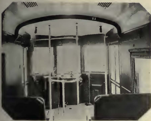
Showing the platform arrangement on the Gary Cars, with all pipes enclosed in cabinet and head lining in vestibule.
