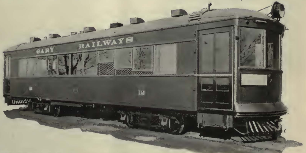
One man, double end cars of the latest type used in Gary, Indiana, on their city, suburban and interurban lines.
