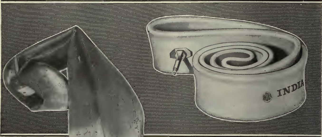
Photograph of a high grade, heavy gauge inner tube of standard make showing the results of heat from high speed service and from aging.
