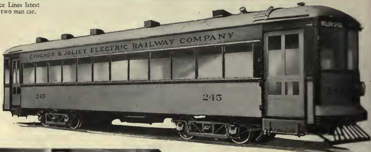
Chicago and Joliet Electric Railway's lightweight inter-urban car. One man, single end operation.
