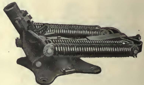
Nuttall US No. 20A Trolley Base Equipped with Timken Roller Bearings.
