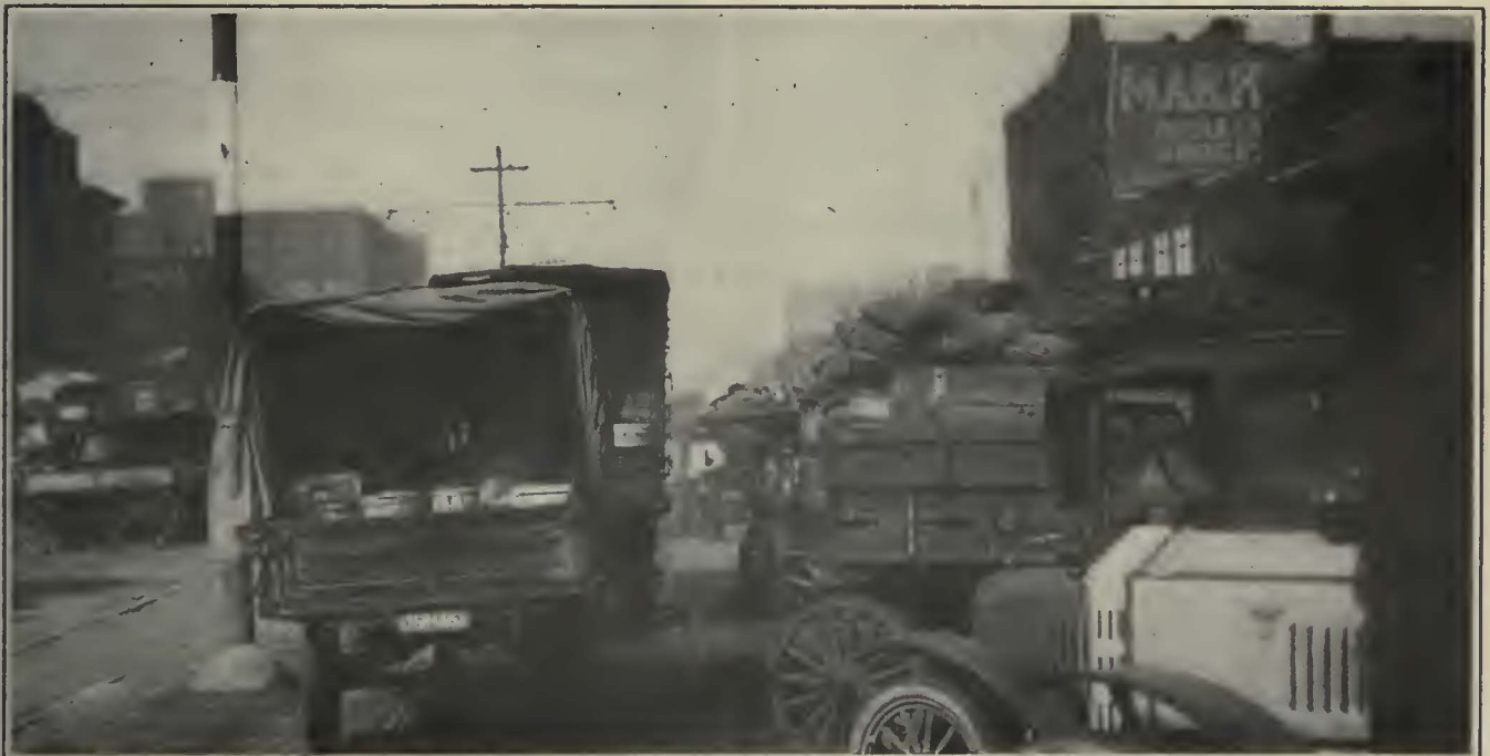
Angle Parking on Narrow Chicago Streets Leaves Only the Track Area Free for Moving Vehicles
