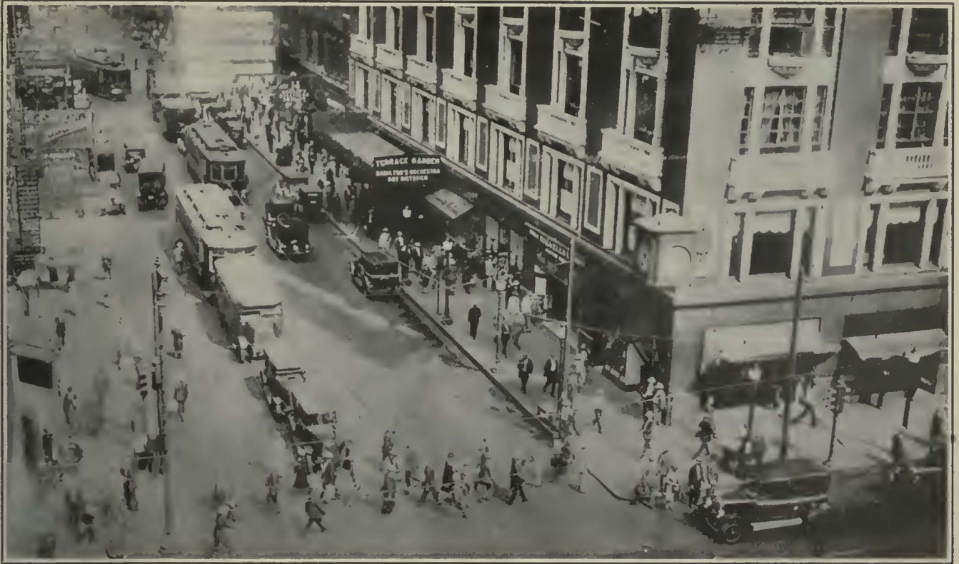
Absence of Loading Zones and Adequate Traffic Regulation Delays the Progress of Street Cars and Their Larger Number of Patrons. In This Typical Instance Two Private Automobiles and a Bus Prevented an Electric Car from Approaching the Corner Despite the Fact that the Curb Lane Was Unobstructed
