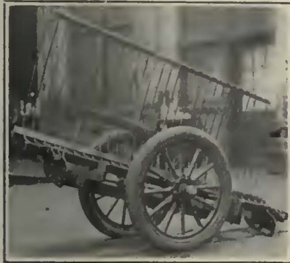
Fender Loaded on Pneumatic-Tired Truck Ready for Transportation
