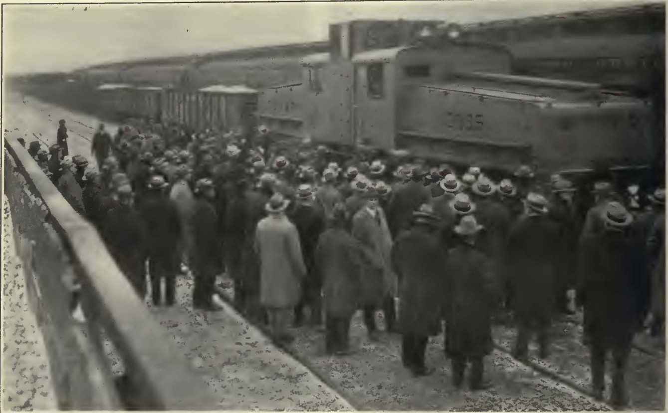
Railroad Officials Watching the Largest Storage Battery Locomotive Start a 1,700-Ton Train Without Taking Slack and Move 100 Ft. in 37.8 Seconds. The M-1 Type Steam Switcher Which This New Unit Is Designed to Replace Could Not Start the Same Train. This Unit Is Now Performing Switching Service in Chicago for the Chicago & Northwestern Railway
