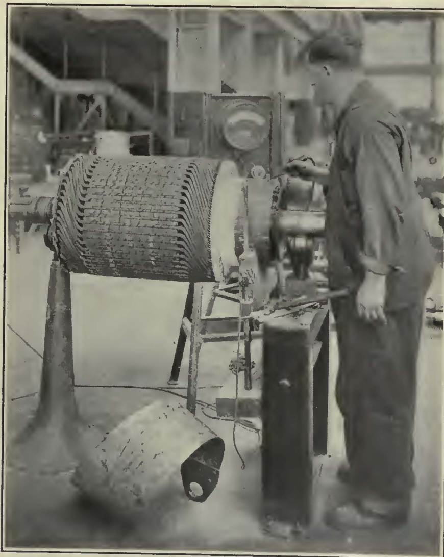
Making a Bar-to-Bar Test in the Department of Electrical Repairs, Brooklyn-Manhattan Transit Corporation
