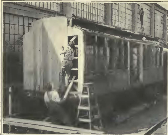
Reconstructing an Old Type Passenger Coach for Use as a Freight Trailer in the Springfield Shops of the Indiana, Columbus & Eastern Traction Company
