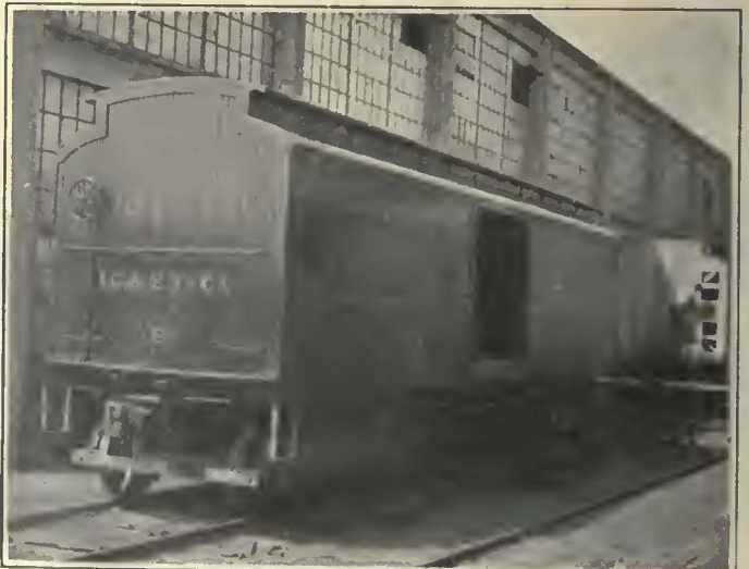
One of the Freight Trailers Just Rebuilt from a Passenger Car. A Few Years ago the I., C. & E. Purchased Several New Light-Weight Passenger Cars to Replace Old Heavy-Weight Wooden Ones
