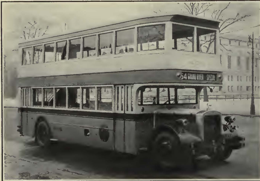
One of the 50 Gas-Electric Coaches Which Are Being Delivered to the Detroit Street Railway System. They Are Designed for One or Two-Man Operation
