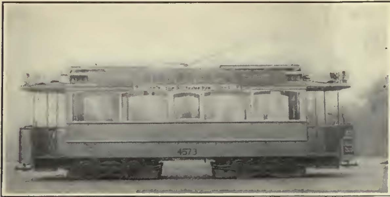
Fig. 2—Double-Truck Motor Car, Weight, 35,200 Lb., Originally Designed for Storage Batteries and Later Used with Overhead Trolley
