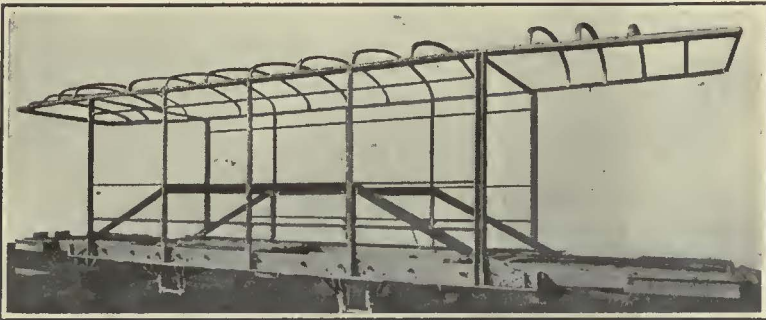
Fig. 12—Framing of the Car Shown in Fig. 11. The Side Sills Are Z Channels
