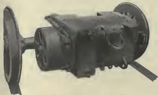
Fig. 10—35-Kw. (47-Hp.) Motor with Drum Brake on the Armature Shaft. This Motor Was Built for Use on the Motor Car Shown in Fig. 9
