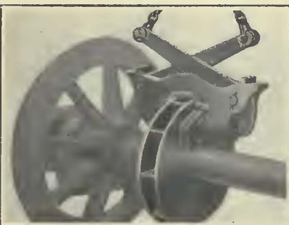
Fig. 13—(At Left) "Tongs" Type of Brake, Used on the New Trail Cars in Berlin. Fig. 14—(At Right) Floor Framing of Berlin Motor Car Equipped with Two Cardan Drive Motors
