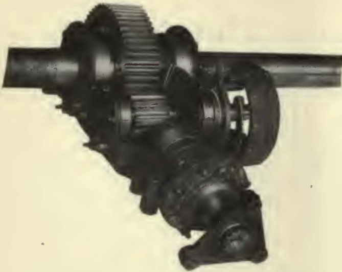
Fig. 17—Cardan-Drive Gearing with Cover Removed, of the type Shown in Fig. 15, Operated in Experimental Service. In This Case the Brake Drum Is on the Gear Shaft and Not on the Axle
