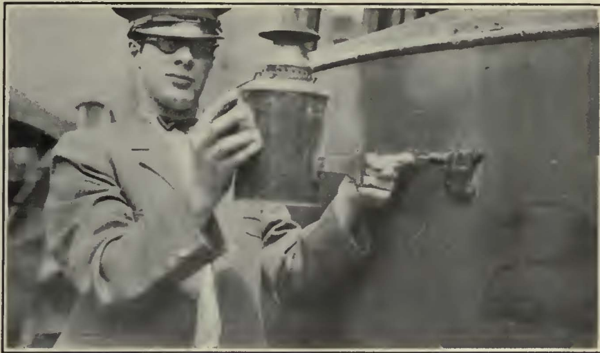
New Style Tail Light Bracket with Spring Bolt Holds the Light in Position Securely
