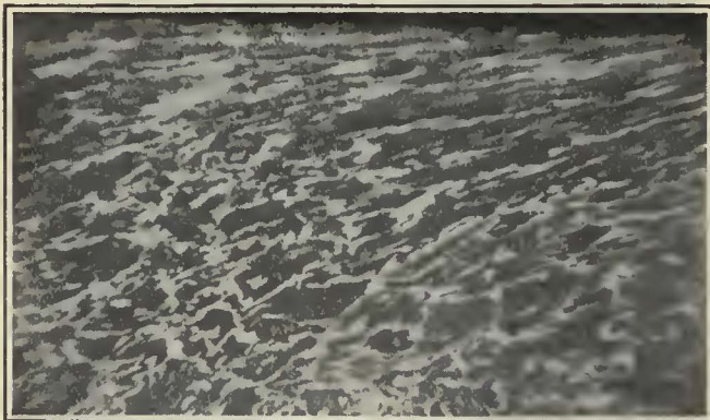
Transverse Cut Through a Rail Head, Passing the Depression—60 Diameter Enlargement
