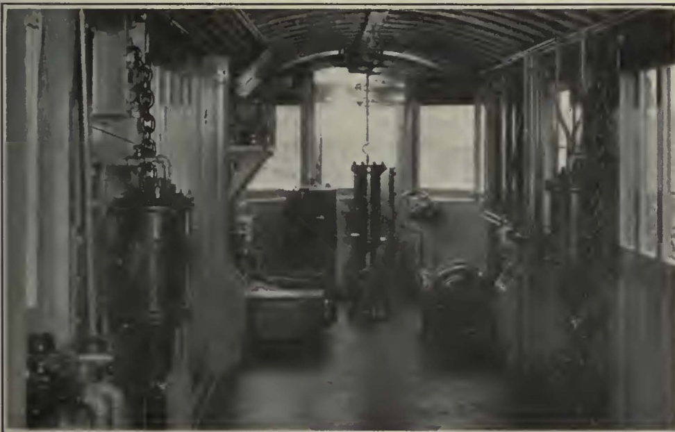
Interior of Snow Plow Showing the Air-Operated Cylinders for the Side Shears Hung on the Side Wall
