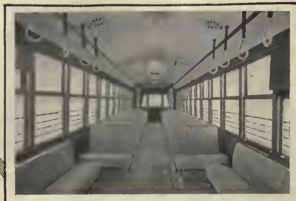
Rubber tile floor covering and center dome direct lighting system also used.
