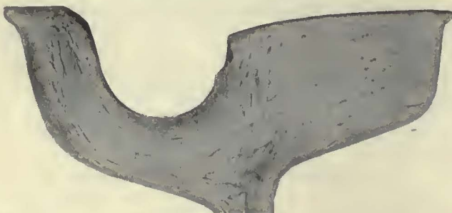
Transverse Cut Through a Rail Head, Showing Distribution of the Displacement and the Side Deformations on the Rolling Surface
