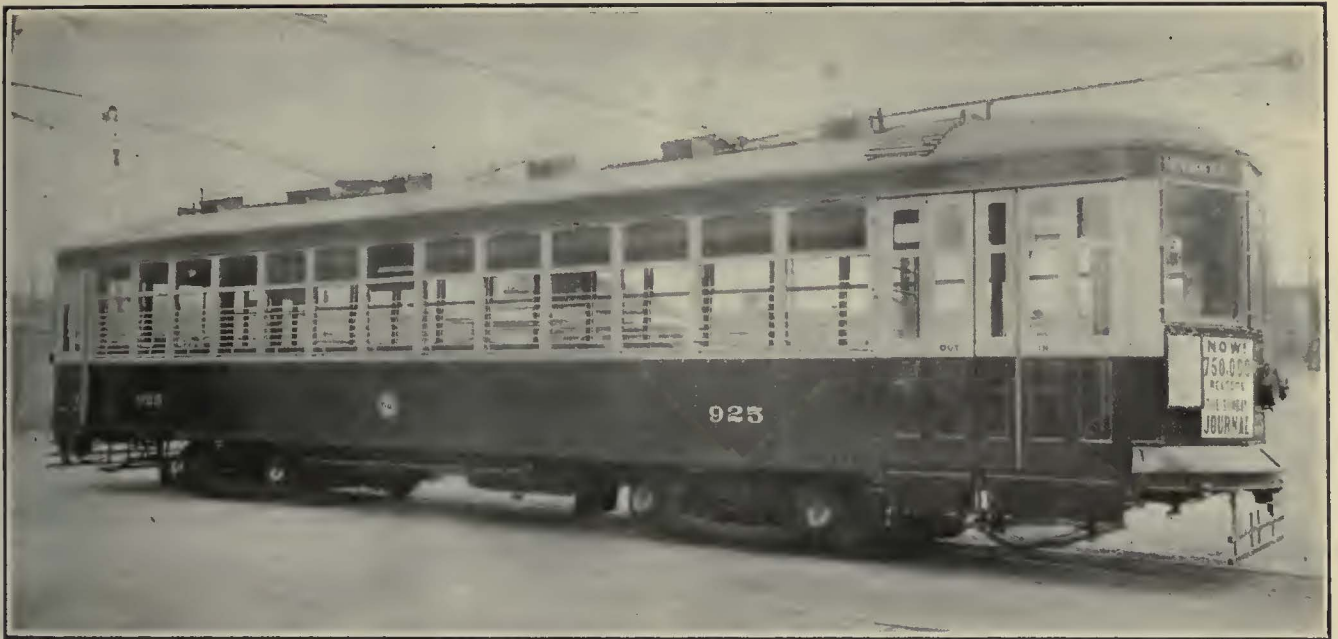
One of 40 New One-Man Cars Built for the Milwaukee Electric Railway & Light Company in the Short Time of 3½ Months. Reduced Width of the Rear Door Gives the Car an Appearance of Added Length
