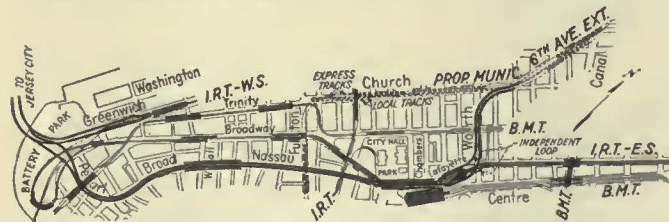
Scheme "G"—Alternate Plan for Physical Connection of North Jersey Transit Line with East and West Side Interborough Subways and Subway of the Board of Transportation Now Being Built in Church Street
