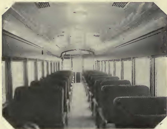
Interior view, showing dome lighting, plush seats, metal sash, etc. Notice on the exterior view, above, that the window guards raise with the windows.
