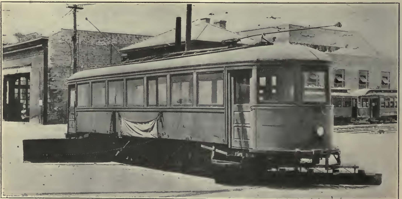
Exterior View of Snow Plow with Side Flanger in Position so that a Space 10 Ft. Outside the Car Is Cleared
