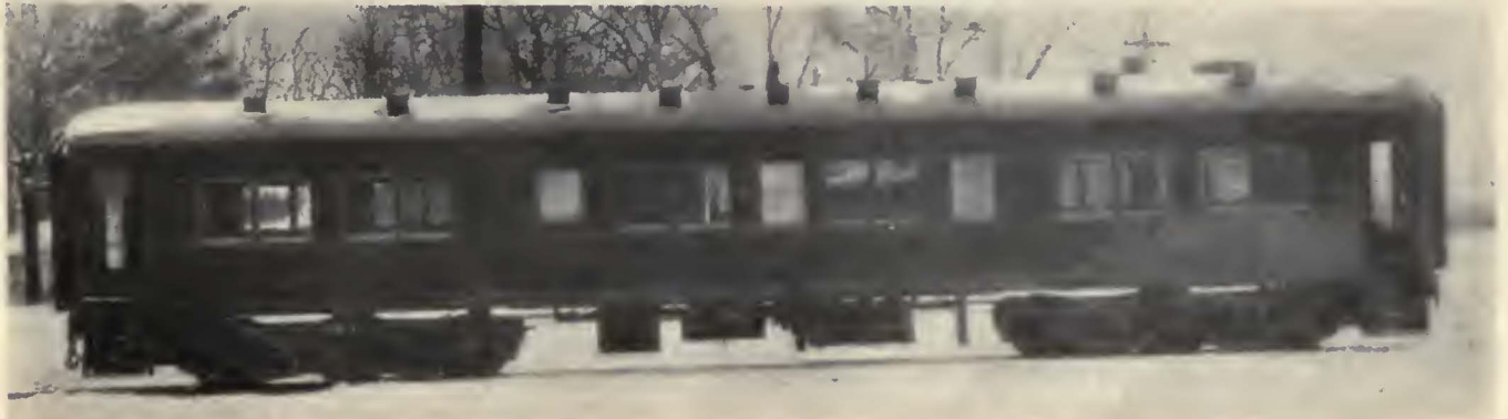
Exterior of South Shore Line's New De Luxe Parlor-Observation Car Showing Six-Wheel Truck Innovation and Glass-Enclosed Observation Platforms
