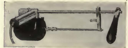
Portable Undercutter, Operating Handle and Other Details
