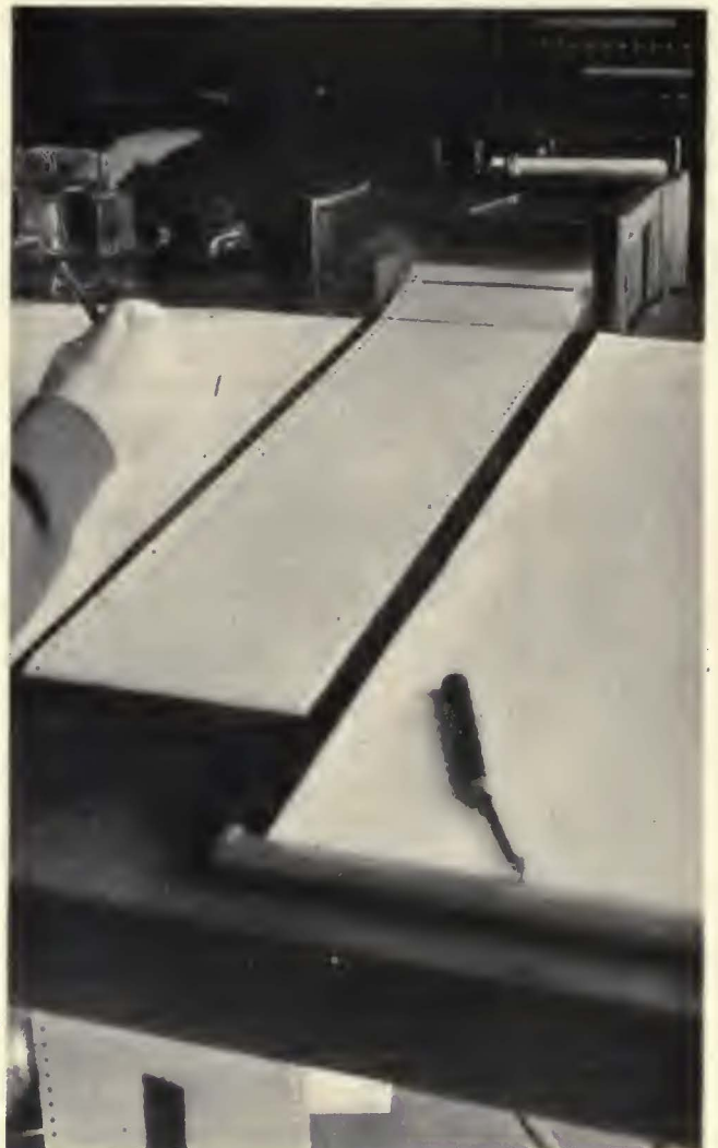
Chart, on Which Are Registered the Headways on Ten Car Lines Operated by the Denver Tramway, Passes Over the Dispatcher's Desk
