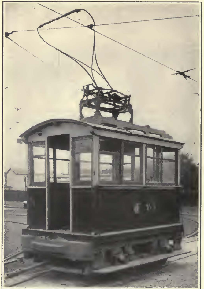
The Bow Collector Is Shown in the Trailing Position on the Car Used for Shifting Trailers
