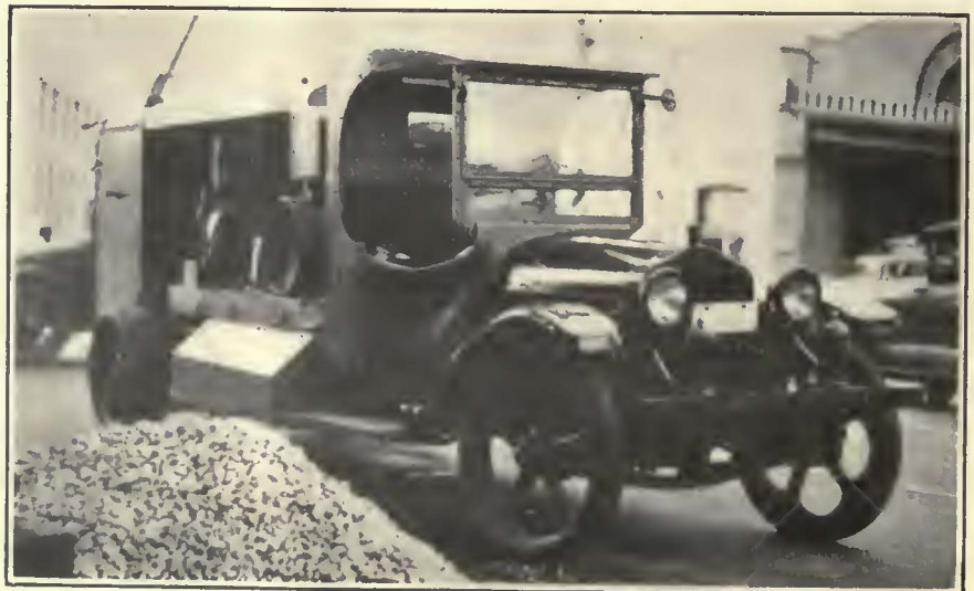
Portable Compressor Outfit Assembled in Bus Chassis by Los Angeles Railway. Boxes on the Sides Hold Various Air-Operated Tools.
