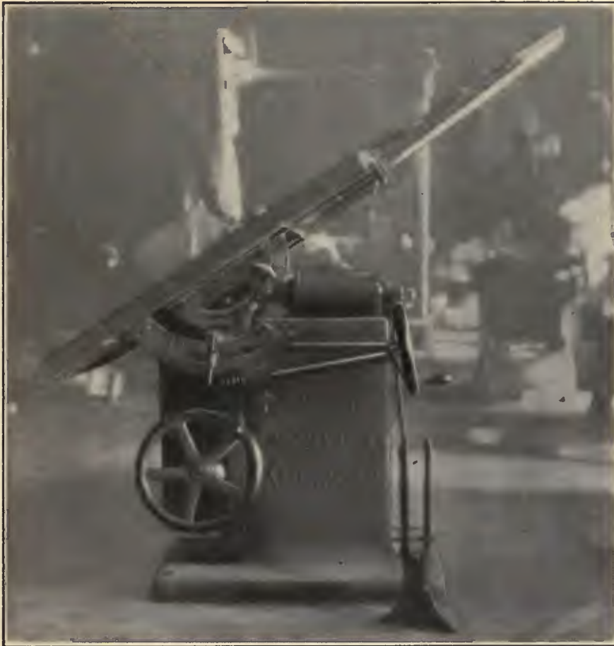
Tilting Table Circular Saw in the Capital Traction Company Shop, with Lumber in Place and Table Set for Angle Cut
