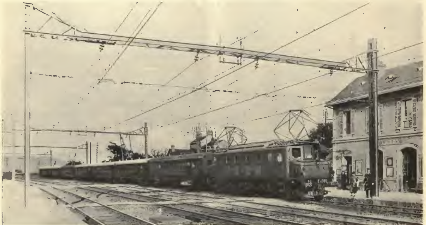
Paris-Vierzon Express on Paris-Orléans Railway Drawn by One of the New 1,500-Volt High-Speed Locomotives
