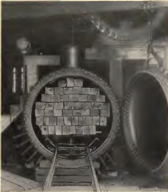
A Load of Ties Has Just Been Run Into the Treating Tank at the Atlanta Creosoting Plant
