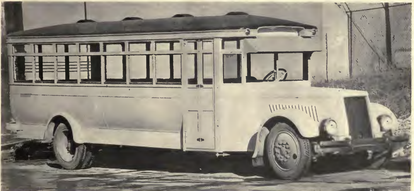
Mack Six-Cylinder Gas-Electric Bus of the Type Ordered for Use in Newark, N. J., and Albany, N. Y.
