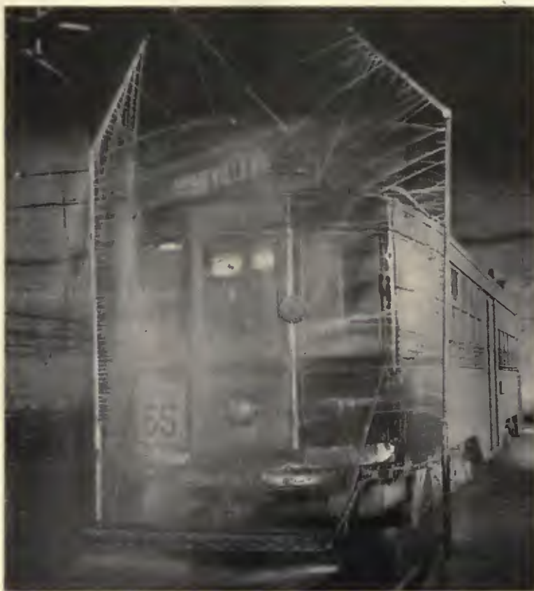
Car Entering the Preliminary Wetting Spray by Passing Between Two 12-In. Upright Pipes Perforated with \frac{1}{4} -In. Holes Spaced 1 \frac{1}{2} In. Apart. By Staggering the Holes the Water Is Sprayed on the Car in Two Directions
