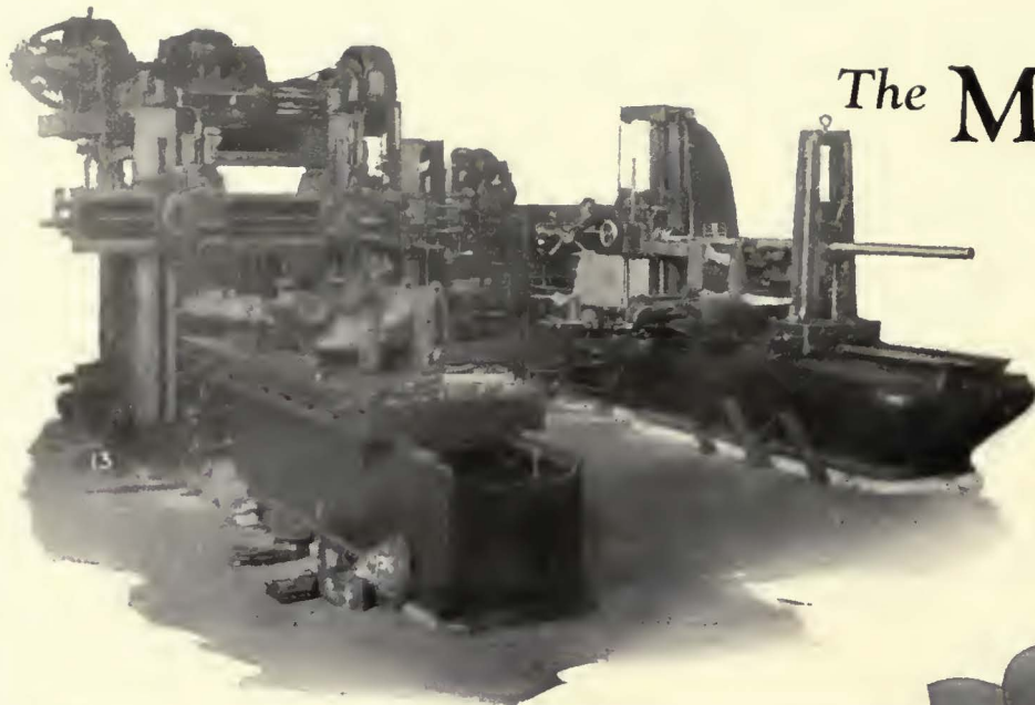
Surfaces of motor shells, gear cases and truck frames are finished on the planer in the foreground, Fig. 13. A motor shell is being rebores in the horizontal boring mill in the rear.
