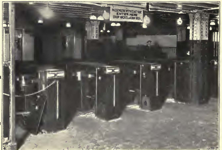
Battery of electric coin turnstiles, collecting and registering each individual fare and passing individual to train platform. Users—B-M-T, Phil. R. Tr., Pub. Serv. Ry., Boston Elevated.
