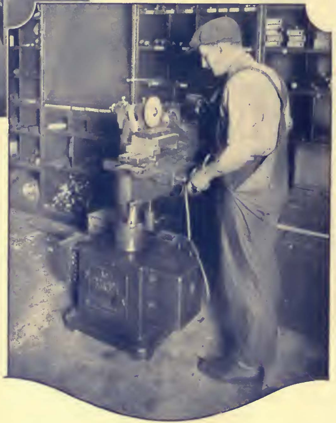
Above— Grand Rapids Drill Grinder. Self-contained motor drive.
