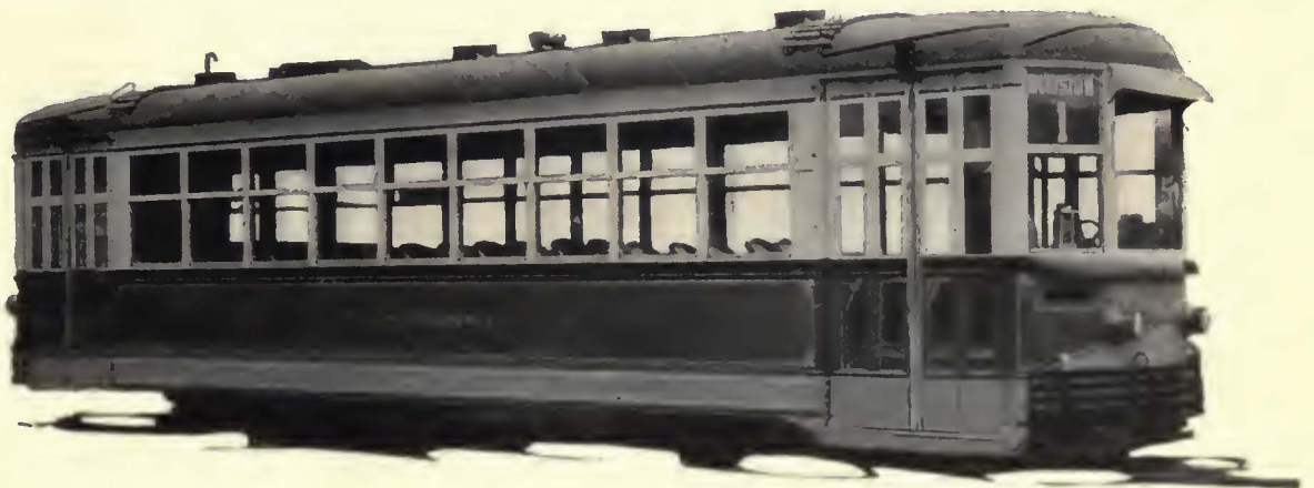
One of the Grand Rapids cars utilizing HASKELITE roofs and interior linings and PLYMETL side panels.
