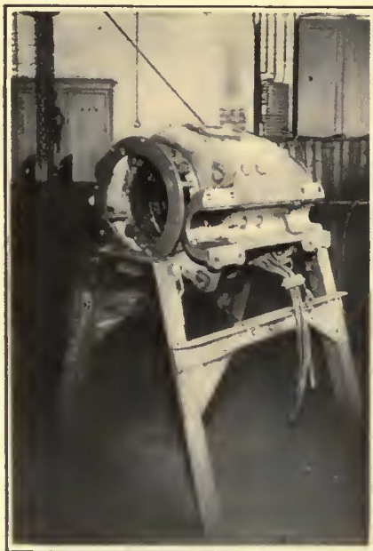
Motor repair stand
