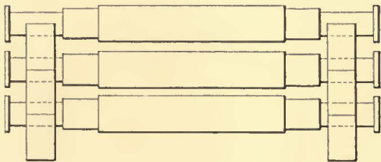
Method of stacking axles with wood blocks used in Richmond, Va. At right, detail of grooved block for axle storage
