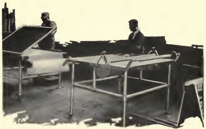
Printing arrangement and device for impregnating Hunter sign cloth with oil to make it impervious to water. This is necessary to prevent buckling and wrinkling
