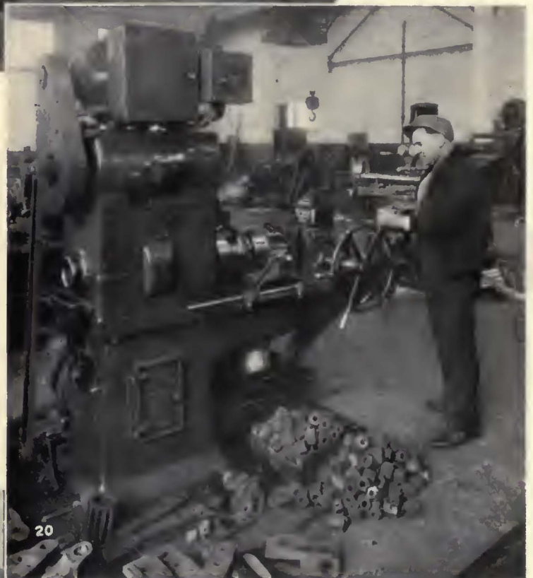
Truck bolts, turn buckles and special nuts are threaded and tapped in the 2½-in. bolt cutter, Fig. 20.
