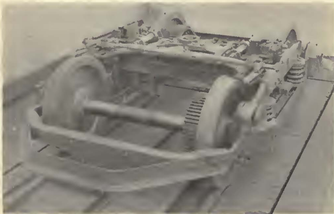
One of the two end trucks before mounting the motors
