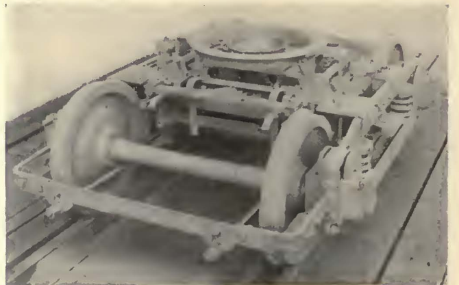
Center pivot truck without motors but supporting two inner body ends and connecting drum
