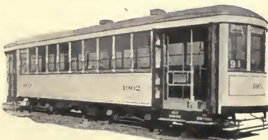
The Montreal Tramway car shown above was built by the Canadian Car and Foundry Co., Ltd., with PLYMETL side panels.
