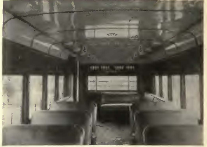
At the rear a sizable well is provided to accommodate passengers leaving by the automatic rear door
