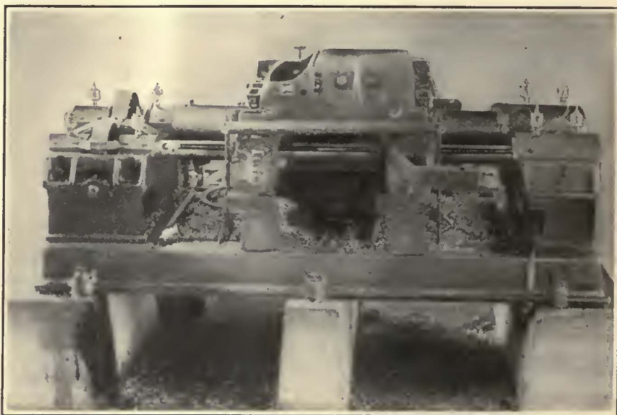
Motor cases being reconditioned in Los Angeles have openings for axle bearing and armature bearing bored on double-end horizontal boring machine
