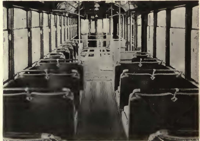
Interior view of experimental "aluminum" car as exhibited during Cleveland convention, showing twin seat arrangement. For exhibit purposes a portion of the floor at the front end was cut away to show the aluminum alloy framing
