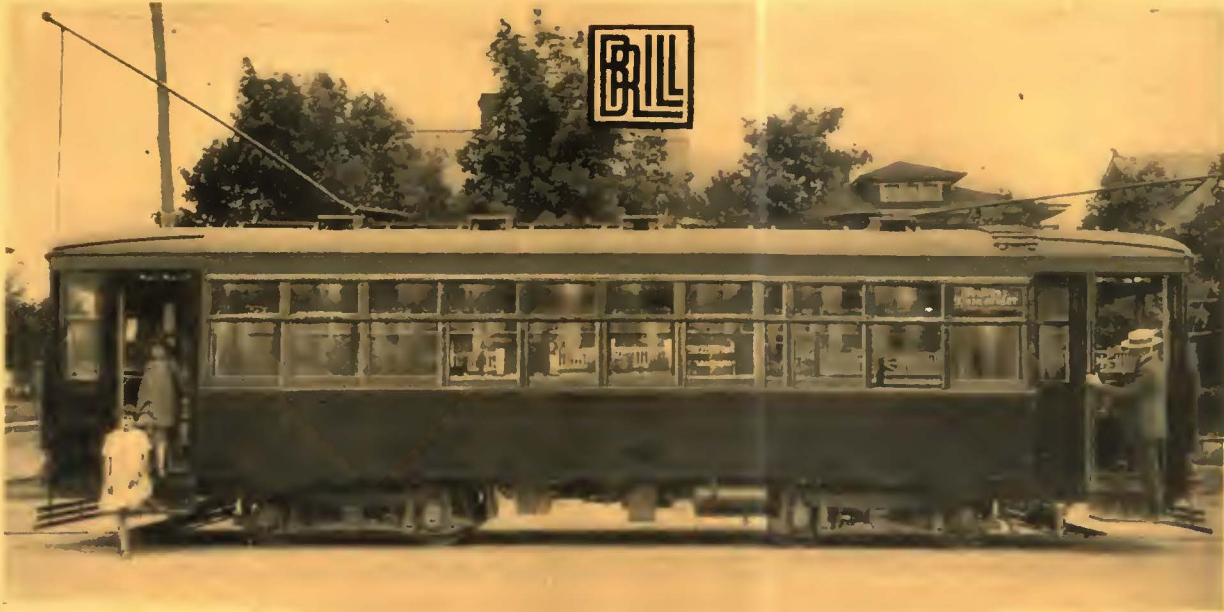
Roanoke's new cars have platform automatic treadles operating rear exit doors in one-man operation.
