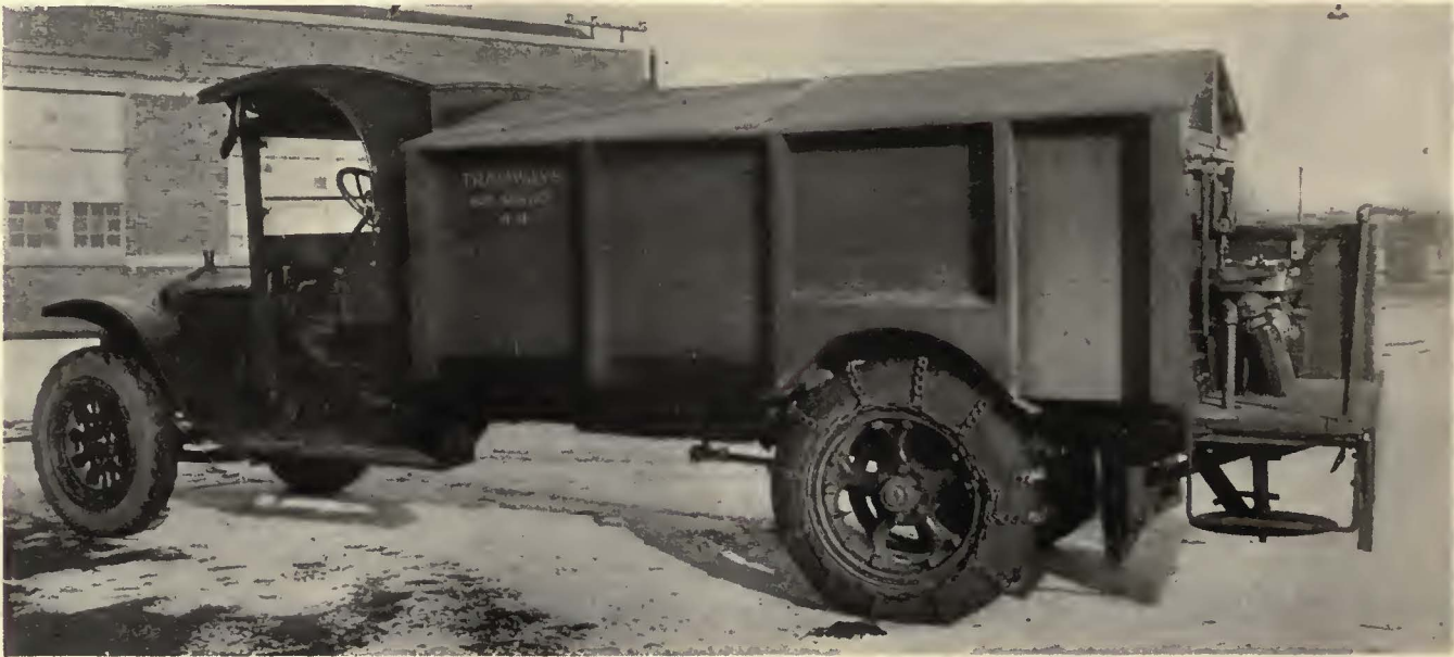
Sand-spreading truck as used on bus routes by the Montreal Tramways
