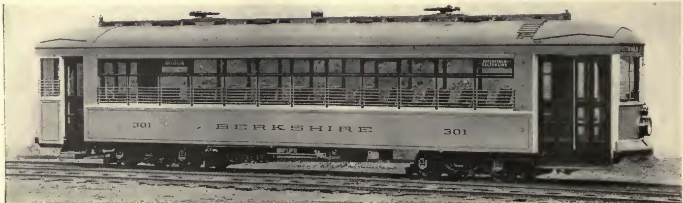
Type of double-truck interurban car recently delivered to the Berkshire Street Railway, Pittsfield, Mass.
