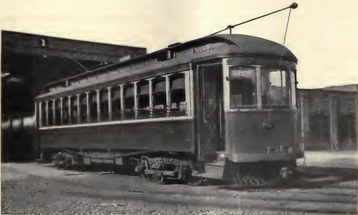
High-speed, multiple-unit cars of the "Shore Fast Line" have been improved in appearance by the installation of sheet steel over the old wood side sheathing
