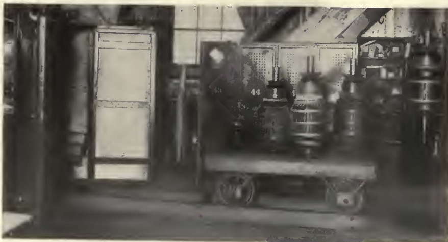
Convenient type of armature truck used for handling armatures between dipping tanks and into oven
