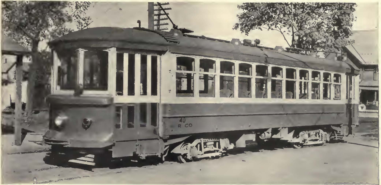
The exterior of one of the 32 cars rehabilitated in Williamsport. Dash floodlighting is in conformity with the new cars recently purchased
