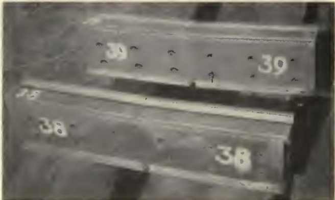
Standard joints Nos. 18, 19, and 38 with \frac{3}{4} -in. x 36-in. fish plates on 9-in. grooved girder rail failed at an average load of approximately 274,440 lb.
