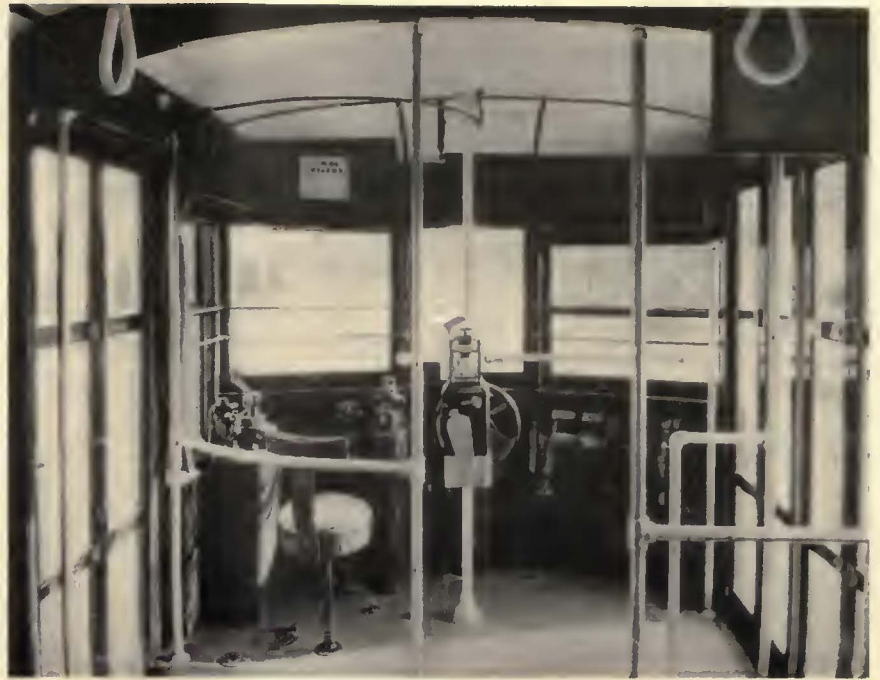
Front platform showing control equipment of the new Virginia Electric & Power Company's cars, five of which were delivered late in March by the American Car Company of St. Louis. These cars were immediately put in service on the Port Norfolk and Pinners Point line
