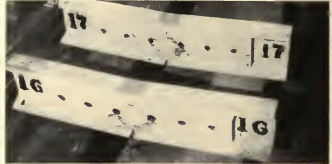
Joint on 7-in. tee rail without base or fish plates broke at 177,500 lb. on 20-in. span
