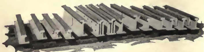
Some of the special welded rail joints made by the Eastern Massachusetts Street Railway and tested in the Riehle machine at the Massachusetts Institute of Technology
