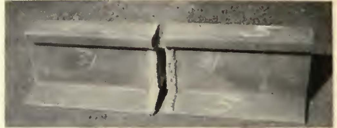
Joint on 7-in. tee rail without base or fish plates broke at 177,500 lb. on 20-in. span
