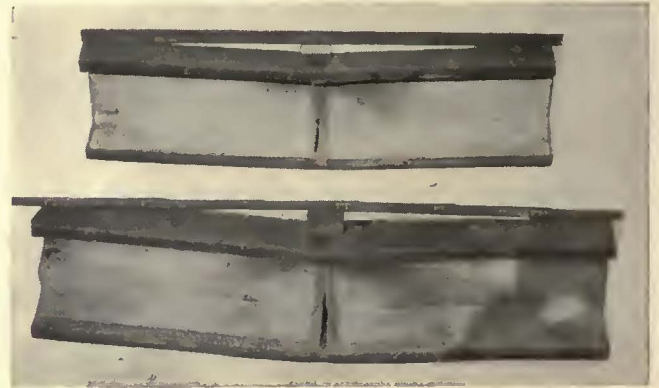
Two joints on 7-in. tee rail with 7-in. x 28-in. x \frac{3}{4} -in. base plates carried maximum loads of approximately 360,000 lb.
