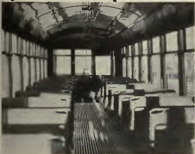
The new Charlotte cars are roomy and airy. They are arranged for operation by one man or two men
