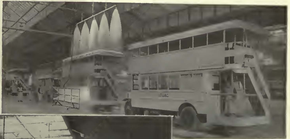
The daily cleaning and inspection includes (1) vacuuming the inside, (2) spray washing, (3) hose washing, (4) inspection
