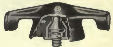
O-B Lock Hanger—Span Type Correct alignment and an absolutely tight joint are achieved. The customary looseness where ears are backed off to secure alignment is avoided by means of the steel spring washer inside this O-B hanger, which eliminates all play. Cat. No. 11062.
