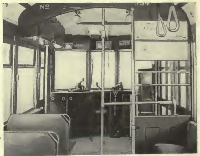
An inclosed cabinet conceals controller and piping, making for a clean platform
