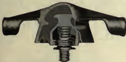
O-B Spring Lock Hanger—Span Type Here is a device which takes the last "hard spot" out of the overhead line and affords a quietness and smoothness of operation heretofore unobtainable. An efficient coil spring between the stud and the hanger body absorbs the impact from pounding trolley wheels. Cat. No. 14532.
