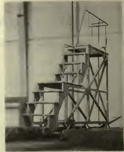
Movable ladder used for car inspection in carhouses of Berlin Surface Lines
