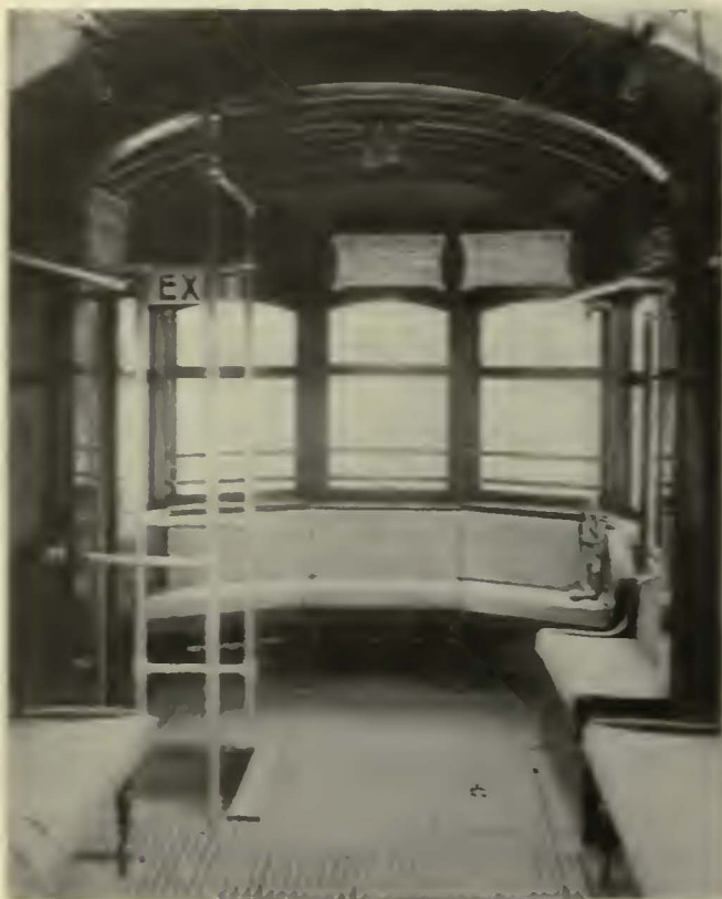
View of rear platform of converted units, showing, at right, wheel which controls special back-up device
