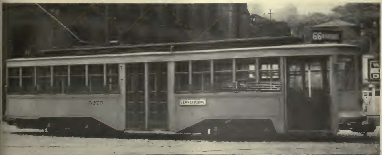
The chair car ready for service. Note the low floor of the car
