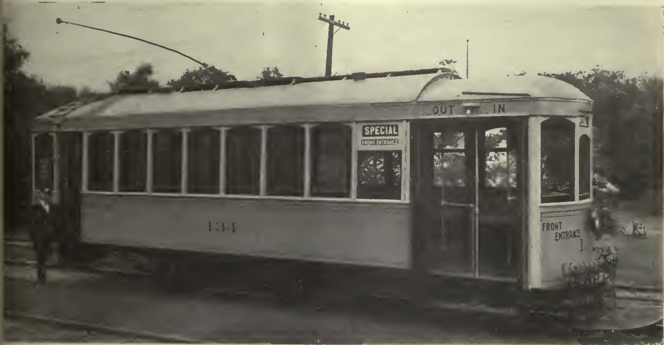
Seven of these one-man safety cars have been turned out of the shops of the London Street Railway, London, Ont., Canada. They were converted from two-man, single-truck units
