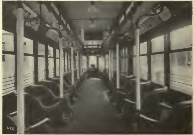
A rear view showing the seating arrangement of the chair car, the stanchions and the one-level floor
