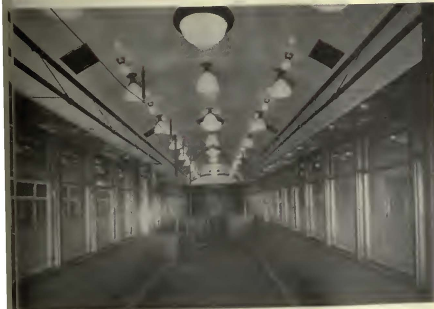
Interior of Cleveland Railway car equipped with four lighting systems on separately controlled circuits
