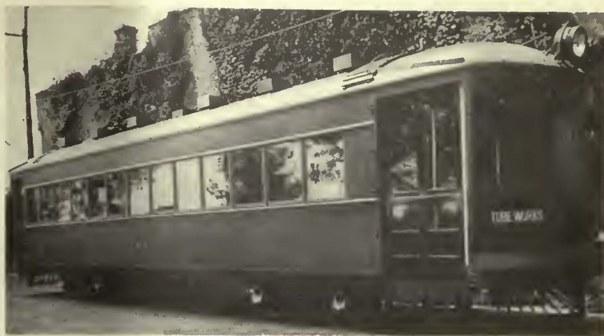
The low vestibule rail in line with the side belt rail carries out the streamline appearance
