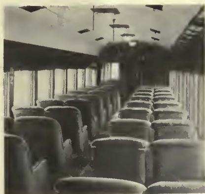
Interior of one of the units showing the rotating, bucket type seats
