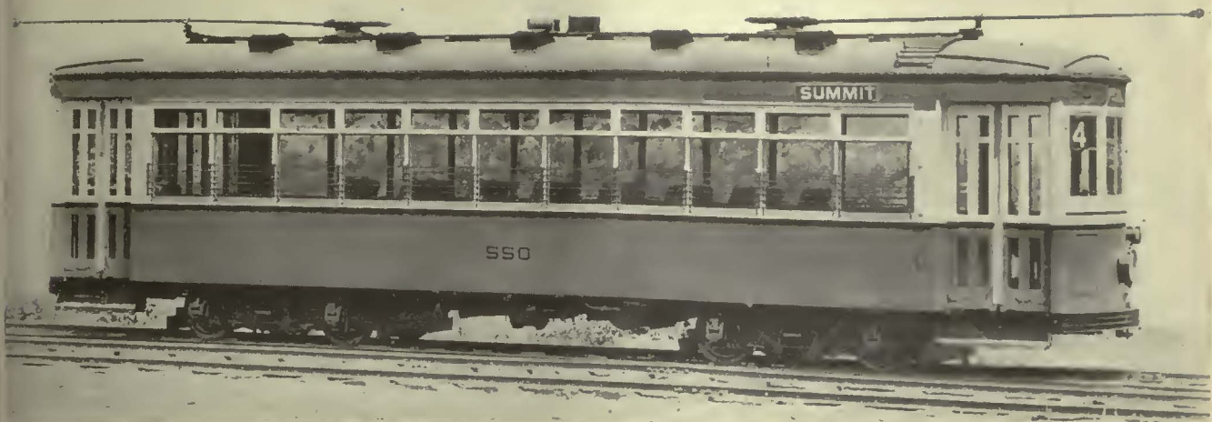
Exterior view of new light-weight city-type cars which were placed in service by Worcester, Mass., Railway Aug. 9. These are almost identical with the Springfield cars
