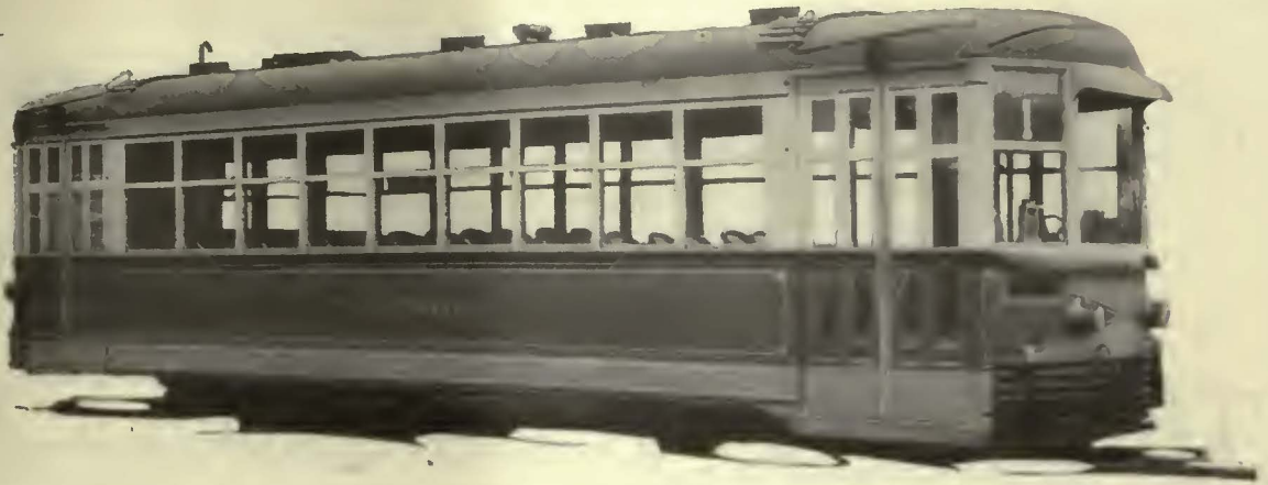
One of the Grand Rapids cars utilizing HASKELITE roofs and interior linings and PLYMETL side panels.
