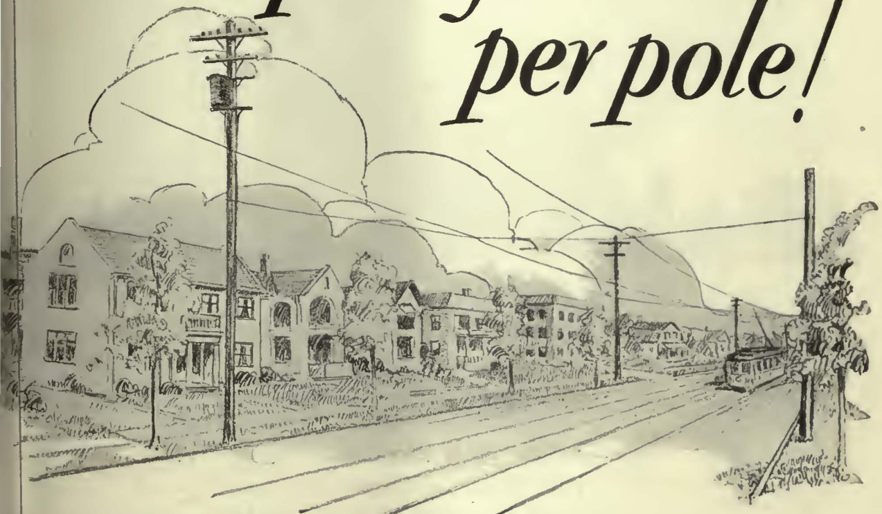
Amcreco creosoted southern yellow pine poles on a Georgia Power Company line.
