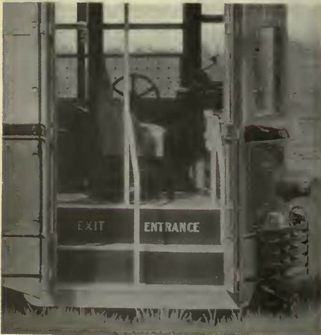
Deep-cushioned adjustable seat for operator, showing also the easy entrance and exit of car
