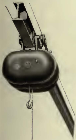
All working parts of this hoist are fully inclosed
