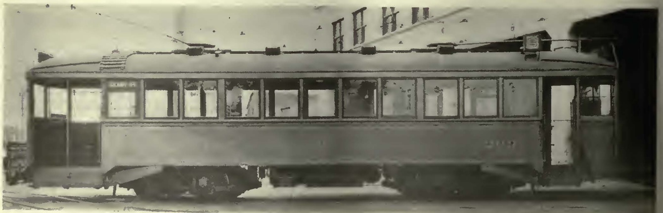
Exterior appearance and specifications of new 50-passenger, semi-steel units for Municipal Railway of San Francisco, ten of which were ordered recently. These are similar to the fifteen units delivered in May
