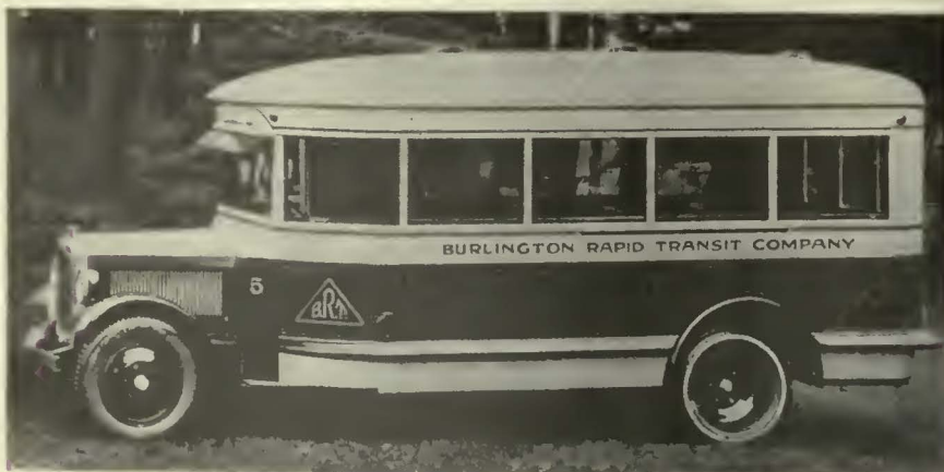
Twenty-one passenger street car body on Graham chassis powered with six-cylinder engine
