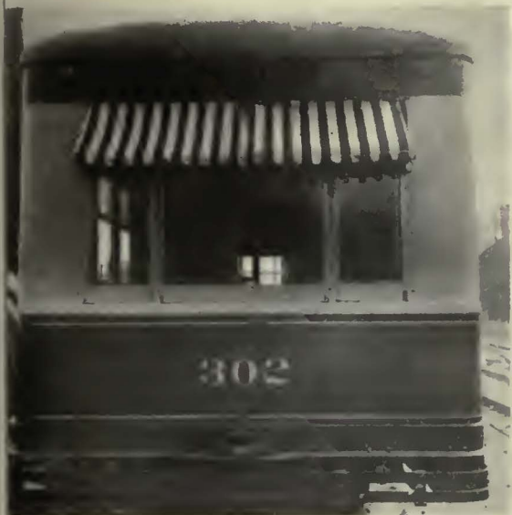
At left, view showing the observation type rear end with wide center window of Rockford cars. At right, interior view showing the one-level floor and the deep-cushioned individual type seats. Note the absence of dome ceiling lights
