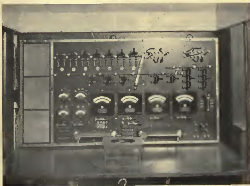
Signal test board used in shops of Philadelphia Rapid Transit Company
