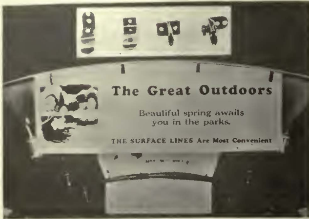
Special clips made in the company's shops are used to support two ceiling cards in each car
