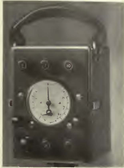
Portable watt-hour meter with temperature compensation features
