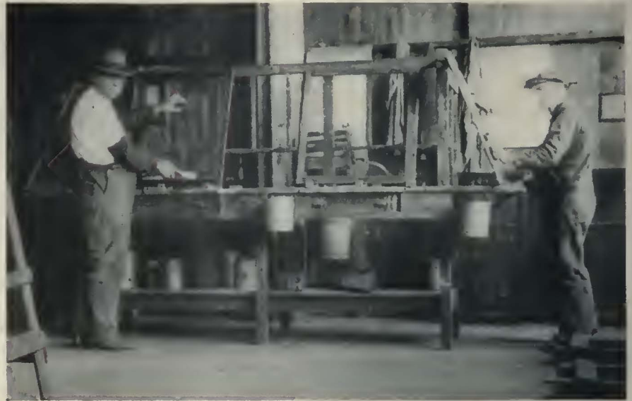
This table, with a rack in the center, facilitates the cleaning of car window sash
