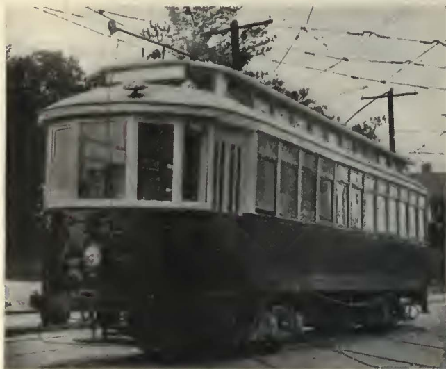
This old car has been fitted out for instruction purposes. The floor has been cut away to show the operation of the machinery. The wiring, air valves and other parts are also visible
