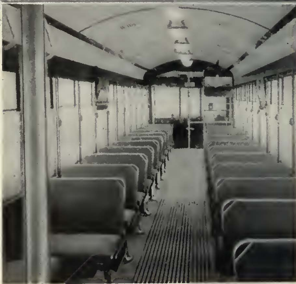
The most recent type of one-man car in Milwaukee includes many features for passenger comfort and safety. The lower view shows the interior of recent one-man city cars with center lighting, wide aisles and comfortable seats
