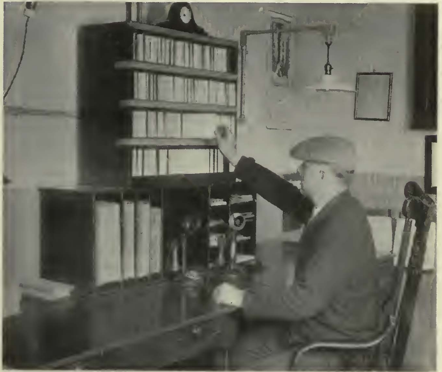
Inspection card rack located in carhouse foreman's office containing last inspection record of each car
