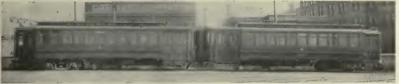
These three-truck trains in Milwaukee have proved very efficient for handling rush-hour loads economically
