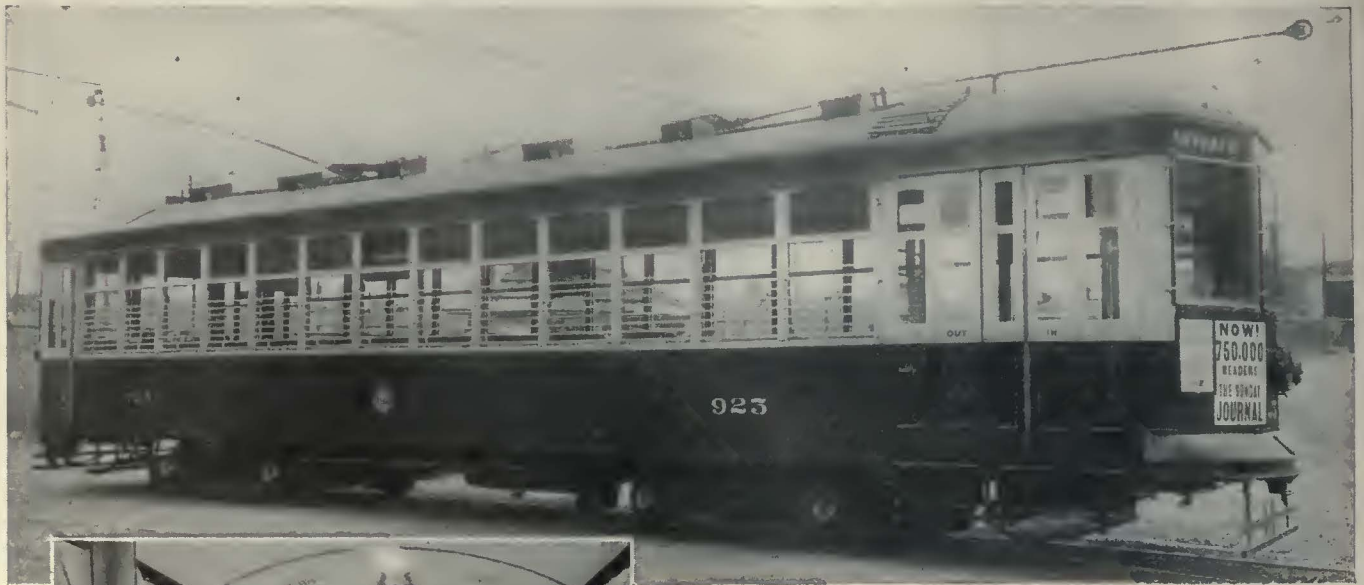
The most recent type of one-man car in Milwaukee includes many features for passenger comfort and safety. The lower view shows the interior of recent one-man city cars with center lighting, wide aisles and comfortable seats
