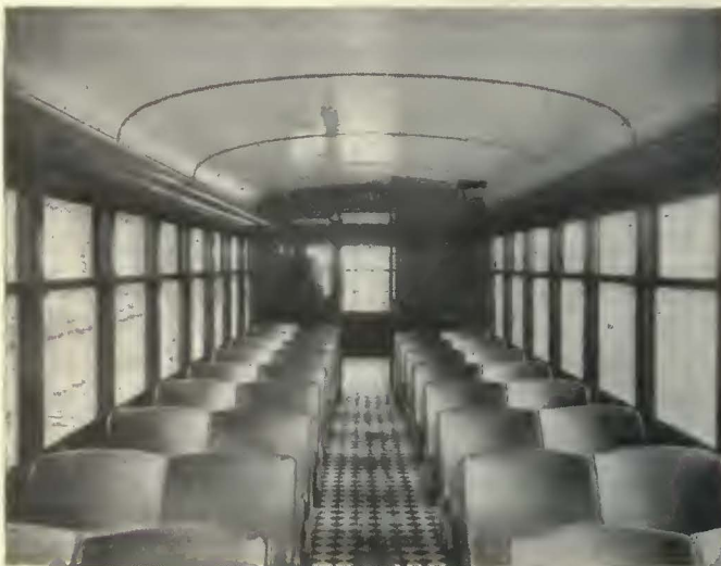
Bucket type seats upholstered in leather and rubber-tiled flooring provide comfort for passengers
