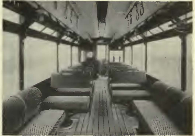
By careful design the lower deck of the new Glasgow tramcar has an interior 9 in. wider than in the previous cars
