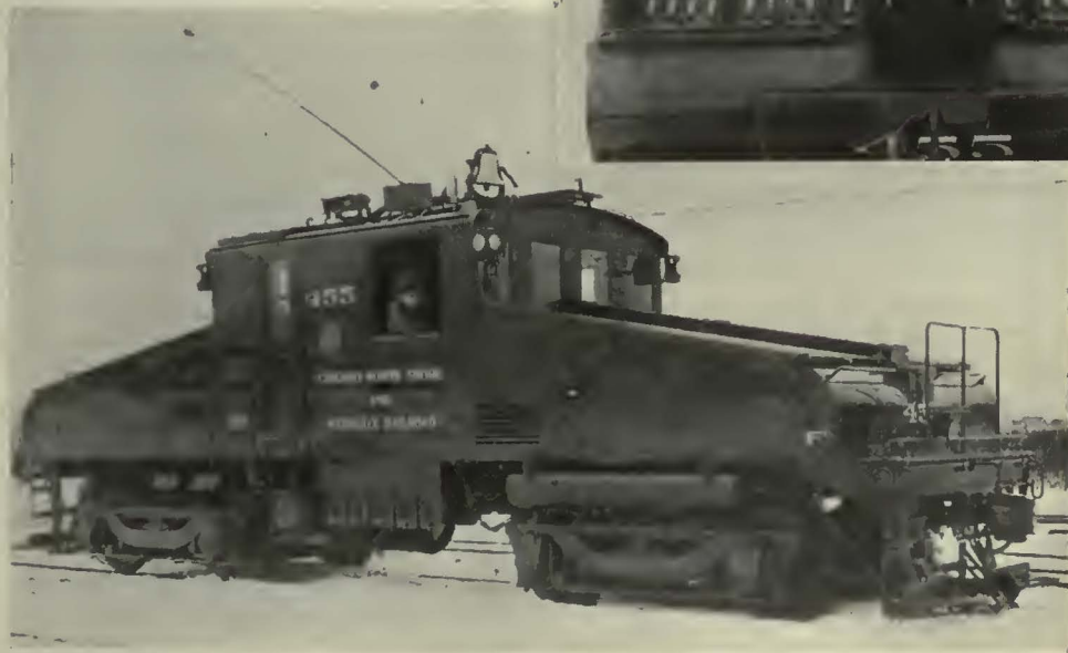
Trolley-battery locomotive—70 tons, 600 volts. The top view shows the battery in place
