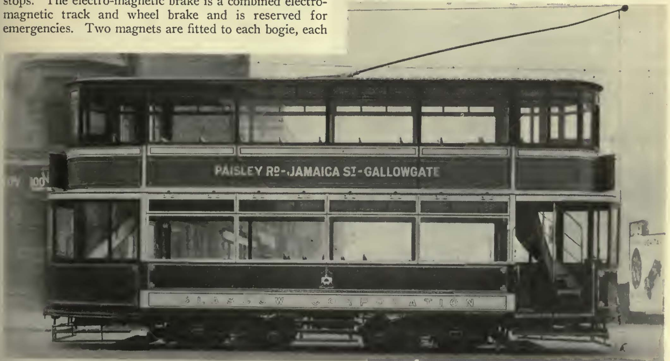
The first of 50 new cars for the Glasgow, Scotland, municipal tramway. These are the first double-truck cars to be used on the property
