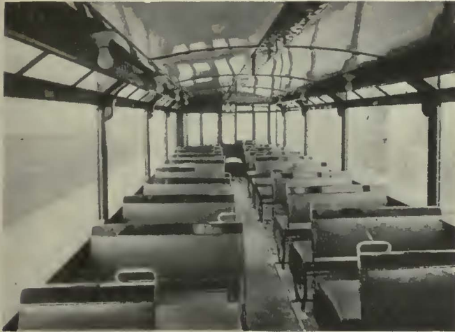
The upper decks of the Glasgow cars are entirely inclosed. This is also an innovation in British design
