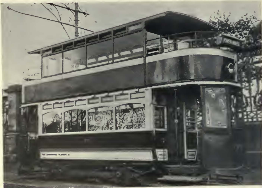
Double-deck car with inclosed upper deck. End-inclosed vestibules are provided
