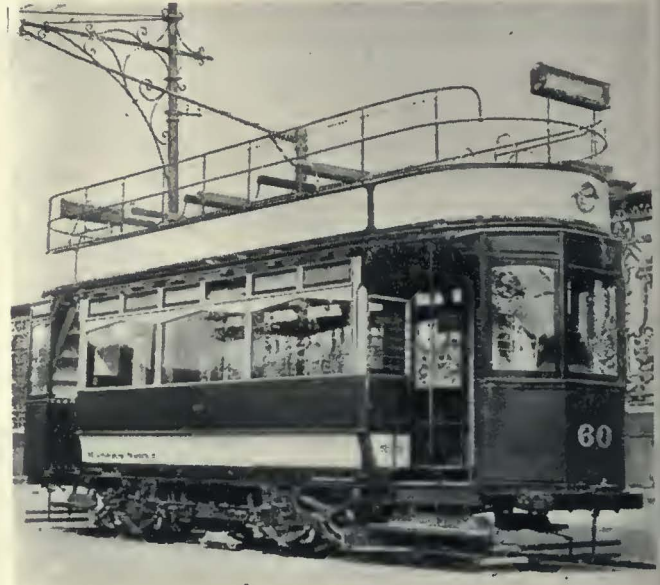
Type of car before remodeling with open upper deck.
