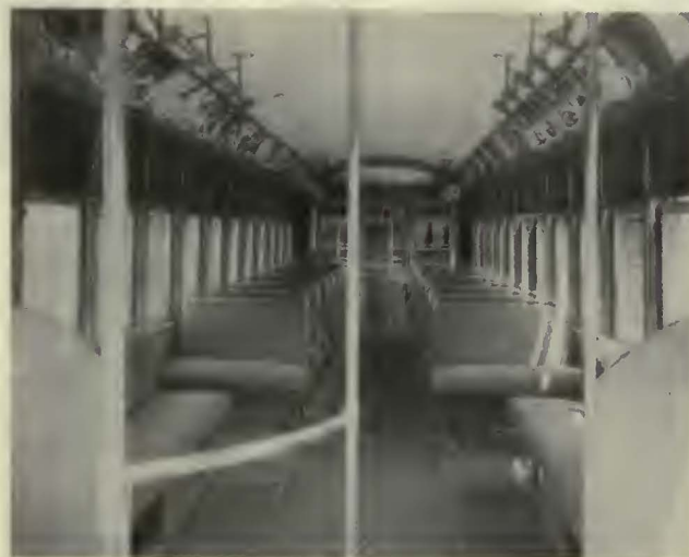
Composition rubber renovable aisle strips and upholstered seats are used in the rehabilitated Kansas City cars
