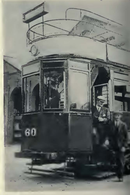
Double-deck car with inclosed upper deck. End-inclosed vestibules are provided
